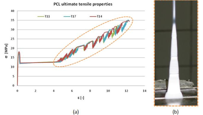
Figure 2: (a) Ultimate tensile properties of PCL and (b) tiered deformation of dog-bone handle.
