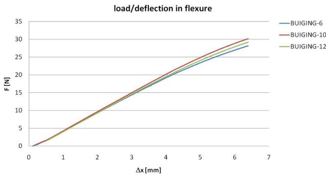
Figure 3: Load-deflection curves for the flexural testing.
