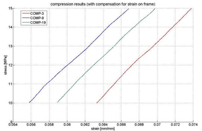
Figure 5: The stress-strain curves for compression, with compensation for frame.
