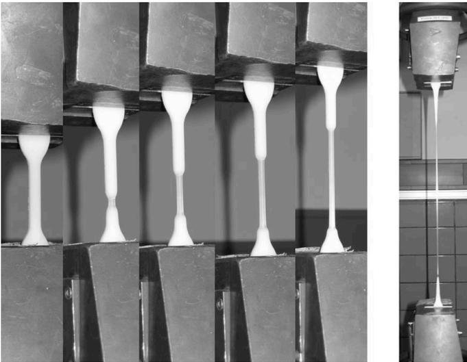
Figure 1: Tensile testing of PCL.
