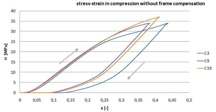
Figure 4: Stress-strain curves for compression (no compensation for frame).
