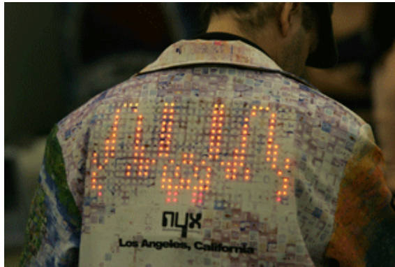
Figure 17 NYX clothing, range of customized jackets with built-in flexible display screens that connect to a Palm OS PDA or smart phone (2006) [40]
