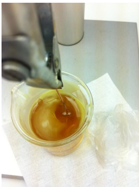
Figure 120 Polyimide dip-coating solution at a humidity of 45%
