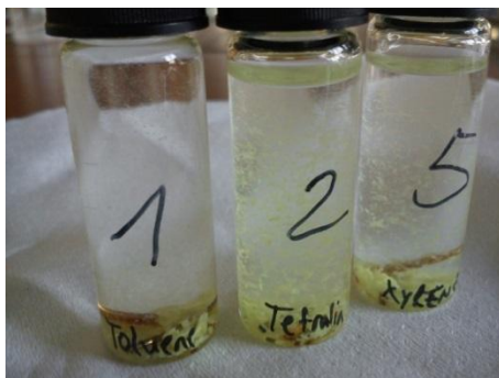
Figure 145 Polyimide resin shows to be insoluble in the solvents toluene, tetralin and xylene (from left to right)
