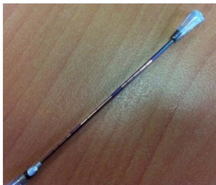
Figure 81 Top-contacts circumferentially evaporated on filament with a length of app. 10 cm
