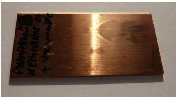
Figure 135 Polyimide layer after drying in vacuum at 60°C for 24 h
