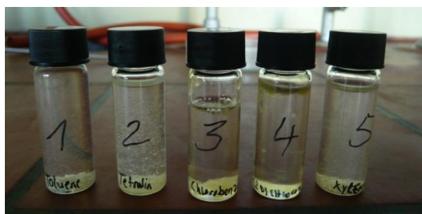
Figure 144 Solubility test of polyimide in toluene, tetralin, chlorobenzene, dichlorobenzene and xylene
