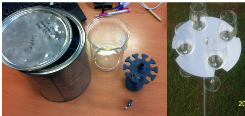
Figure 139 Third generation sample holder (left) following the example of a glass holder (right)
