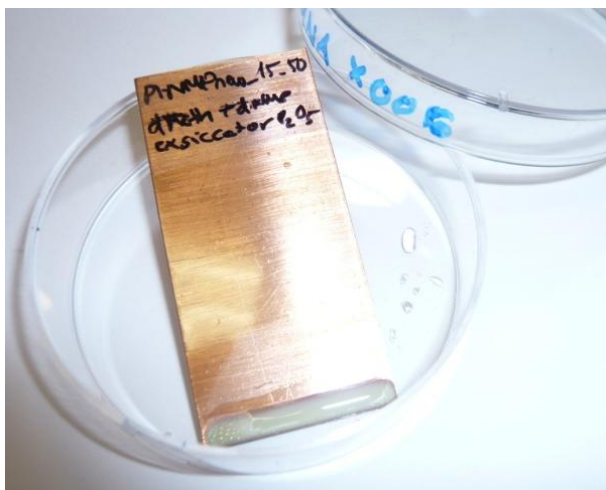
Figure 134 Test on polyimide layer when drying in solvent rich environment
