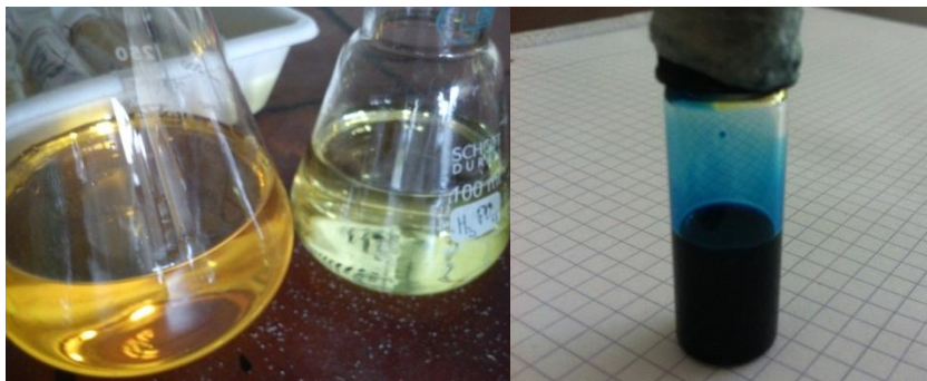
Figure 146 Solution of 2w% TIPS-pentacene in xylene degraded (left) and in toluene stored in vessel with argon gas (right)
