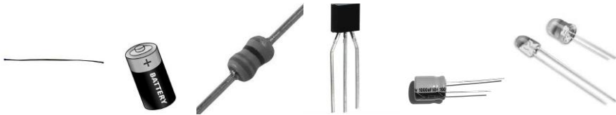
Figure 5 Examples of common electronic components: wires, batteries, resistors, transistors, capacitors, LED (from left to right) [28]
