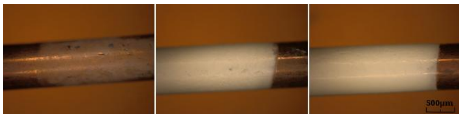
Figure 114 Copper coated PES filament dip-coated with PI/DMF at 50 mm/min with a PI concentration of 10w%, 15w% and 17.5w% (from left to right)
