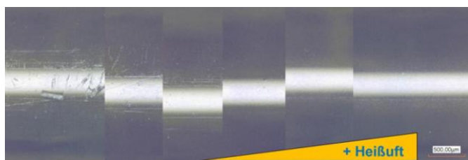
Figure 86 Smoothing effect in treating the ETFE coated HCS glass fibre for smoothing the surface [110]
