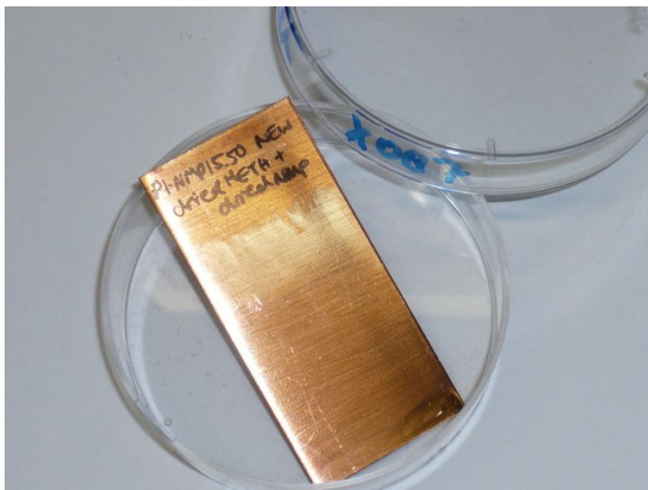
Figure 132 Disrupted polyimide layer morphology on copper plate
