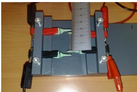
Figure 66 Image of a set up with four flat alligator clamps to make contact (left) and schematic representation (right)
