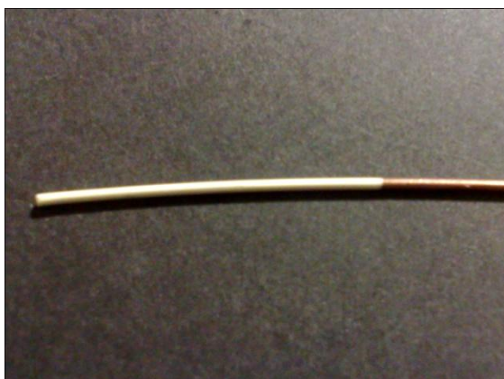
Figure 113 Whitening of polyimide layer on Copper-coated Polyester filament (PI/NMP 12.5w%, 50 mm/min)
