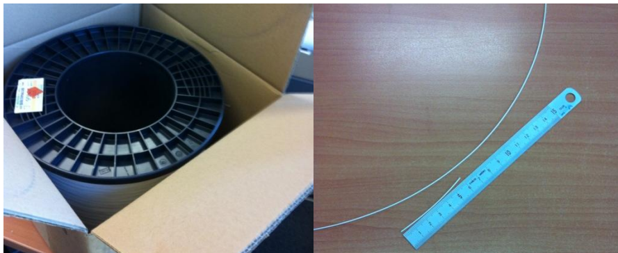
Figure 72 Polyester filament on reel (left) and after removal of the same (right)
