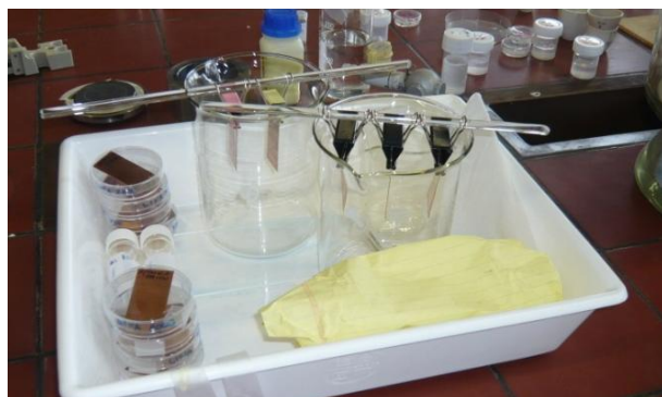
Figure 136 First generation sample holder
