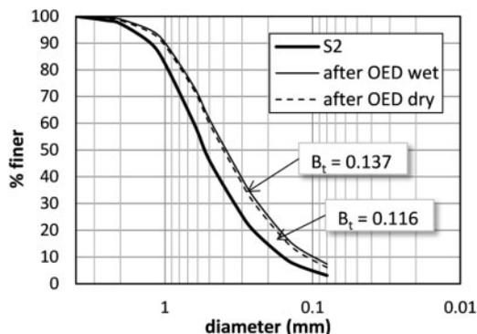
Figure 7. Particle size distributions after oedometer tests on wet and dry S2 sand. The total breakage  $B_t$  in this study is taken as the area between the original PSD and the PSD after testing, for particles larger than  $63 \mu\text{m}$ .
