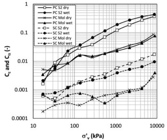
Figure 4. Primary and secondary compression index for wet and dry S2 and Molsand, as a function of vertical stress.
