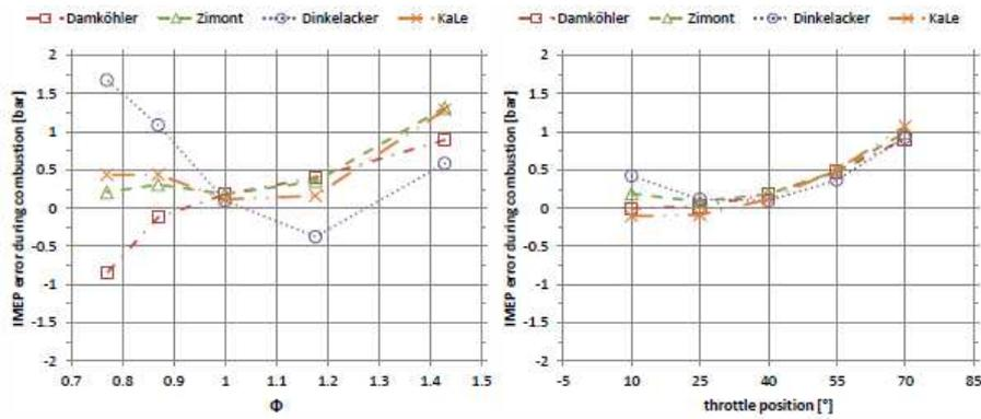
Figure 7. Comparison of  $u_1$  correlations for varying mixture equivalence ratio (left) and varying load (right)
