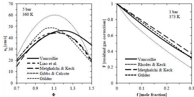
Figure 1. Comparison of predicted  $u_1$  as a function of  $\phi$  (left) and residual gas correction terms (right). 'Vancoillie' refers to the correlation developed in [18]
