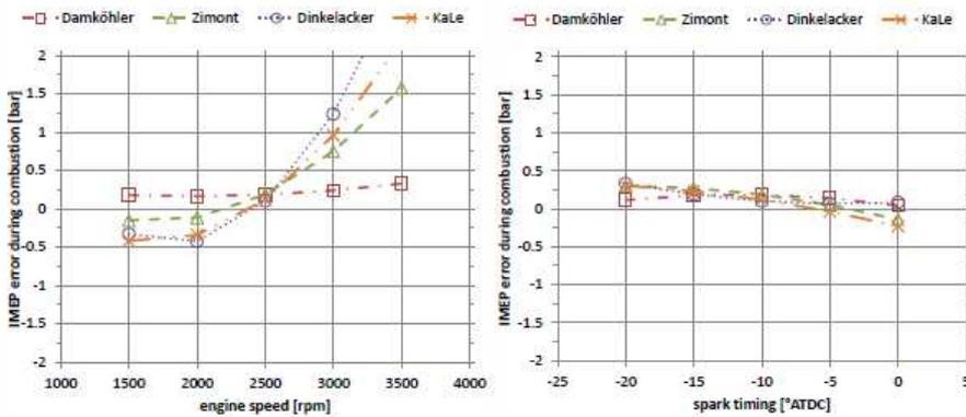
Figure 4. Comparison of  $u_1$  correlations for varying engine speed (left) and ignition timing (right)
