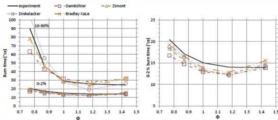
Figure 5. Comparison of  $u_1$  correlations for varying mixture equivalence ratio
