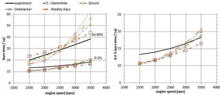
Figure 2. Comparison of  $u_t$  correlations for varying engine speed
