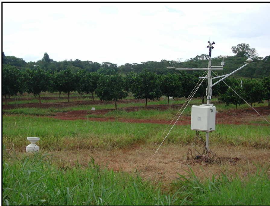
Fig 2.6 Automatic weather station to monitor the orchard microclimate at the trial site at Mazowe Citrus Estate, Zimbabwe. The orchard with four-year-old Navel orange trees can be seen in the background.
