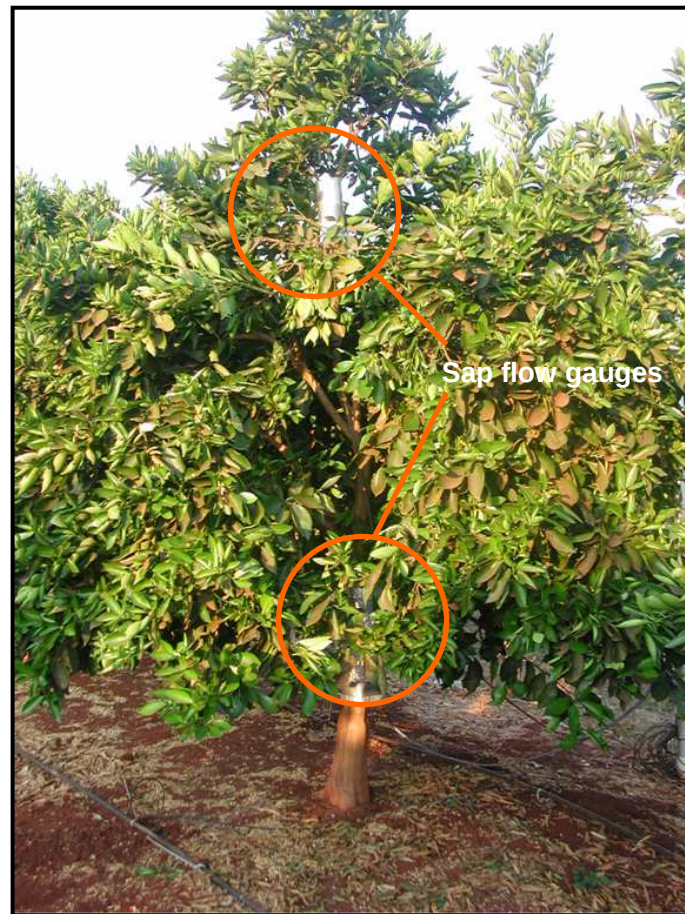
Fig 5.7 Sap flow gauges measuring the stem and the branch sap flow rates on a typical model tree at Mazowe Citrus Estates, Zimbabwe.
