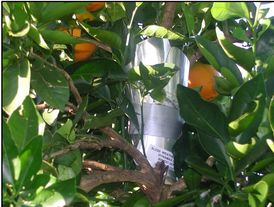
Fig 2.7 Heat balance sap flow gauge (SGB19; Dynamax Houston, USA) installed on a branch of a four-year-old Navel orange tree at Mazowe Citrus Estate, Zimbabwe.
