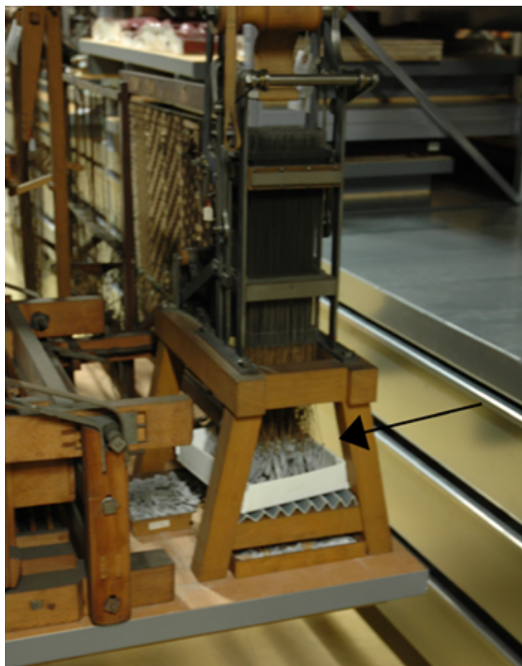
Figure 3.1: Model of the weaving loom by Jacquard . The corroded lead weights are still hanging on their original thread and are indicated with an arrow.
