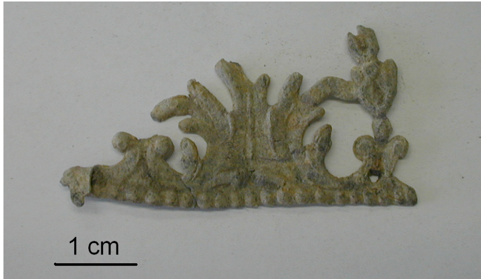
Figure 1.5: General corrosion developed on a lead object. The details of the original object, even though covered by the uniform corrosion layer, remain clearly visible.
