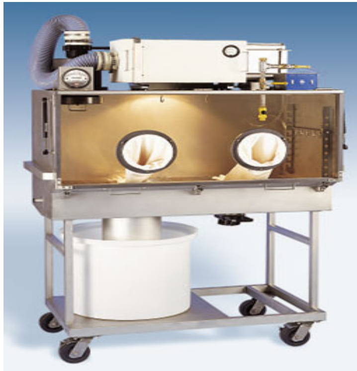
Fig. 4.1. Negative pressure isolators were used for housing the birds.
