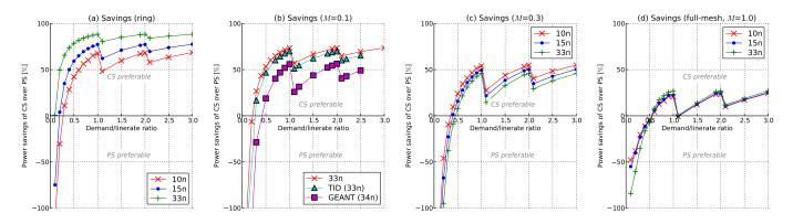
Fig. 4. Influence of the node count on the power savings of CS over PS (for linerate = 10G). Only for sparse topologies (i.e, (a) through (c)) the node count has an influence on the savings. While for a ring topology a higher node count leads to more savings, this is not consistently the case for other sparsely meshed topologies. The apparent deviation of the Géant topology from the general trend is explained in Fig. 5.
