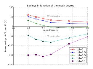
Fig. 7. Influence of the mesh degree and the demand/linerate ratio d/l on the relative savings of CS over PS (for linerate = 10G, and 15-node topologies). For low demand/linerate ratios there is an optimum point where PS is favorable.
