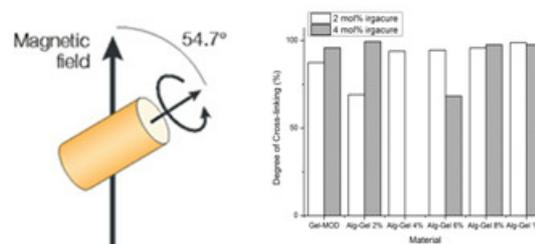
Figure 1: Schematic overview of HR-MAS NMR spectroscopy (left). Cross-linking efficiencies (%) for the various biopolymer derivatives when applying different photoinitiator concentrations obtained using HR-MAS NMR spectroscopy (right).
