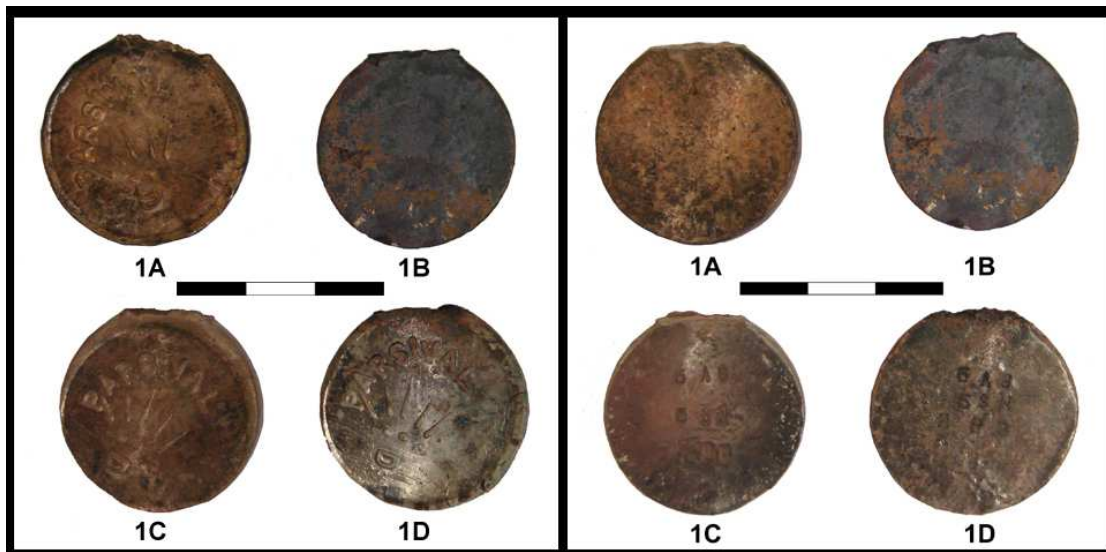
Fig. 105: Visual results (obverse and reverse) of blanks of alloy 1 (5 wt% Ag – 5 wt% Sn – 2 wt% Pb) after different treatments.
