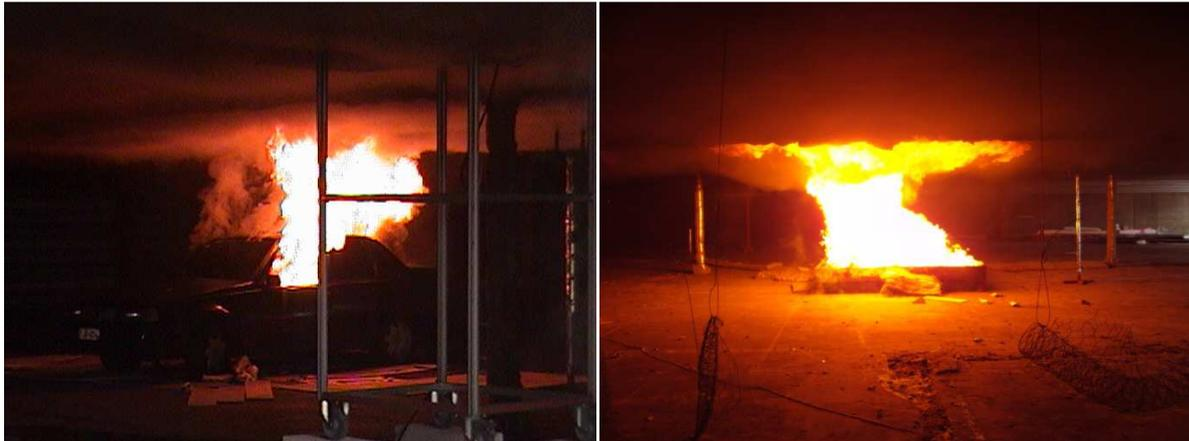
Figure 2. Picture of single burning car (left) and hexane pool fire of 4MW (right). Oncoming air velocity is low.
