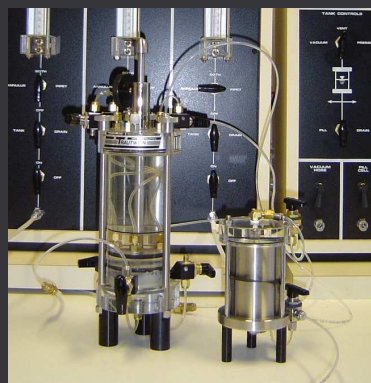
Figure 2. a) scheme of the chemico-osmotic apparatus - b) osmotic cell - c) pump and cylinders
