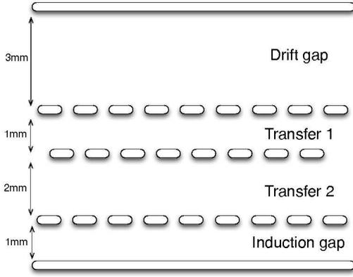
Fig. 1. Gap configuration for the full-size prototype GE1/1\_II.
