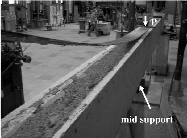
**Figure 15:** Debonding at the mid-support by crack bridging
