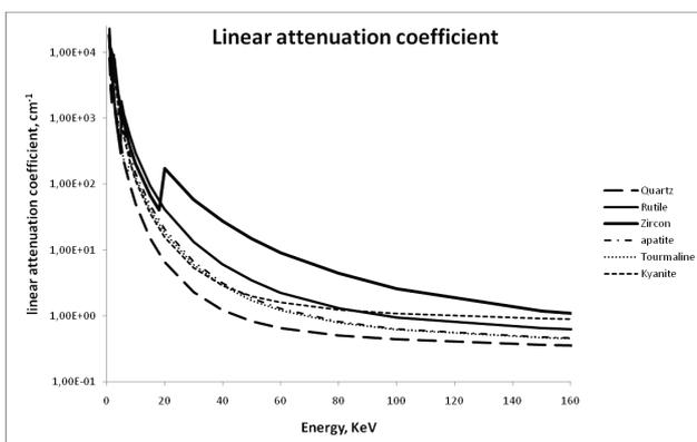
**Figure 12.** Linear attenuation coefficient of the main minerals in the quartzite of Tienen and Wommersom
