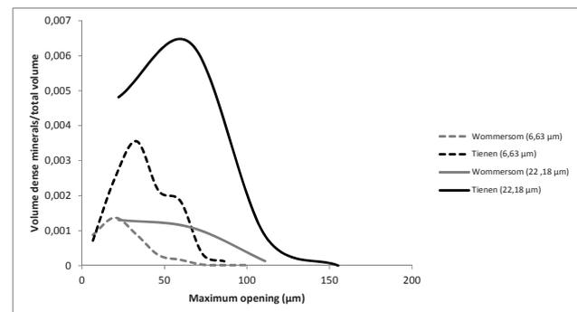
**Figure 13.** Graph of the analysed dense minerals inside the Wommersom and the Tienen quartzite, derived from CT analysis
