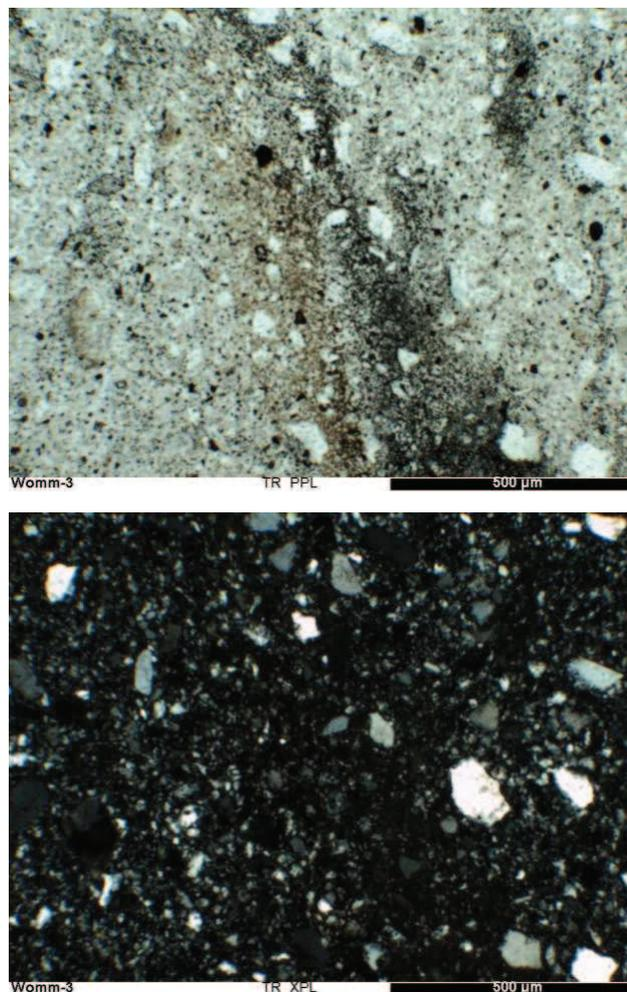
**Figure 4.** Wommersom quartzite under plain light (A) and under crossed-polarized light (B)
