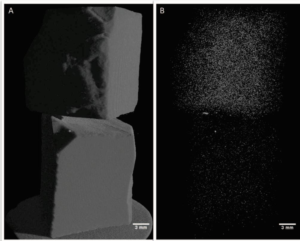
**Figure 11.** A) 3D rendered volume of the large Tienen (top) and Wommersom (bottom) sample; B) 3D rendered volume of the dense inclusions inside the large Tienen (top) and Wommersom (bottom) sample
