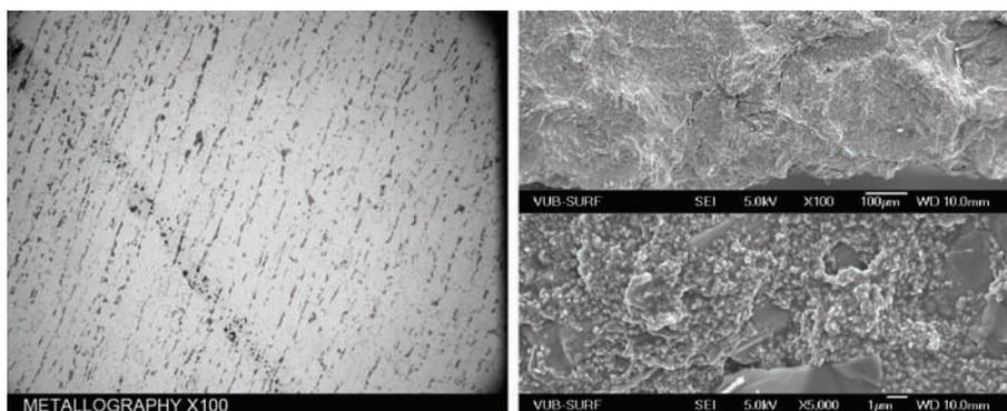
Figure 5-22: (left) Linear structure from metallography of mild steel substrates with magnification  $\times 100$ <sup>31</sup>; (right) more random structure from SEM analysis of failure surface of S235 - Sa3 sample with magnification  $\times 100$  on top and magnification  $\times 5000$  on bottom
