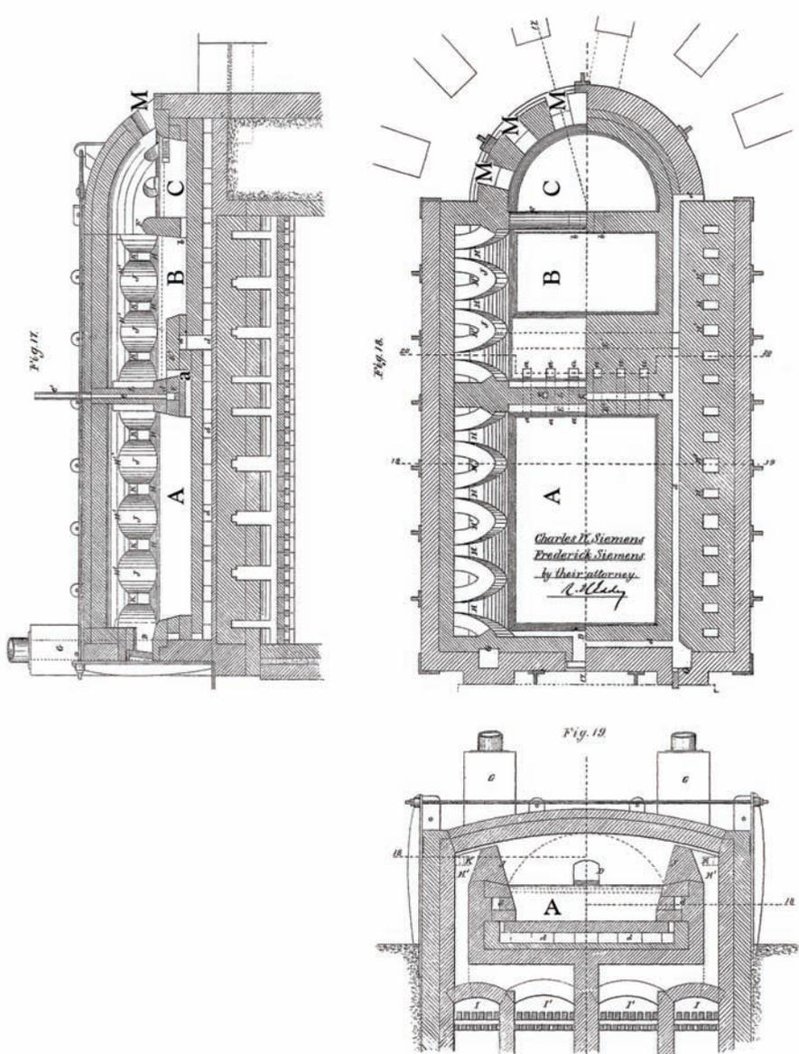
Figure 1-23: Drawing of tank furnace<sup>172</sup>
