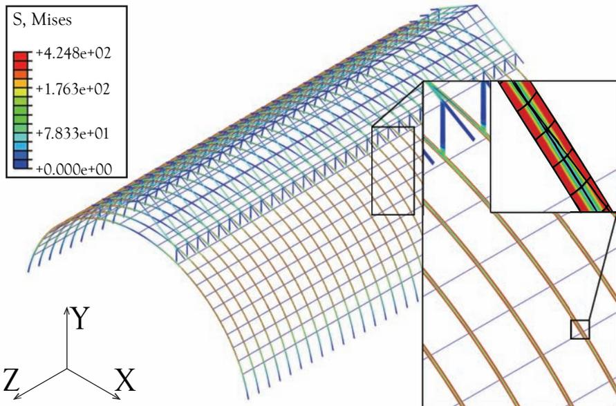
Figure 6-30: Von Mises stresses in iron components for the 4b\_low model under asymmetric perpendicular loading
