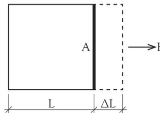
Figure 6-18: Translational stiffness under axial loading
