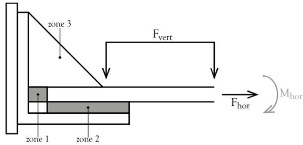
Figure 6-15: Loaded zones of the real connection detail
