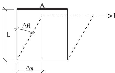
Figure 6-19: Rotational stiffness under shear loading
