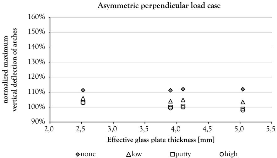
Figure 6-31: Maximum deflection of the arches for the asymmetric perpendicular load case (normalized for 4a\_putty model)
