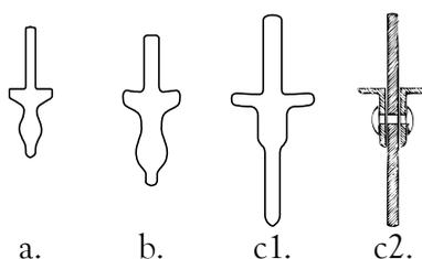
Figure 4-3: Glazing bars used in Kibble
