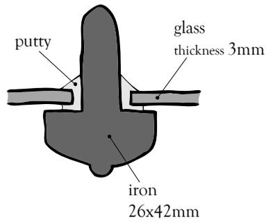
Figure 2-36: The transverse connection at the UCB library: detail as surveyed by the restoration architects before 2003-10 renovation campaign
