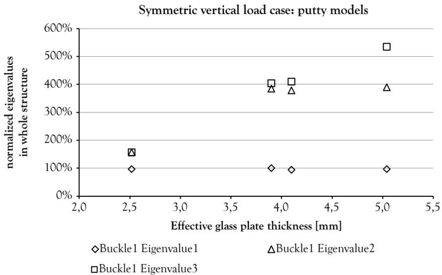
Figure 6-40: Influence of glass thickness on absolute value of eigenvalues of the first buckle step for putty models for the symmetric vertical load case (normalized for first eigenvalue in 4a\_putty model)
