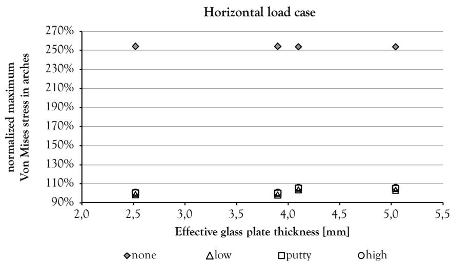
Figure 6-47: Maximum Von Mises stress in the arches for the horizontal load case (normalized for 4a\_putty model)
