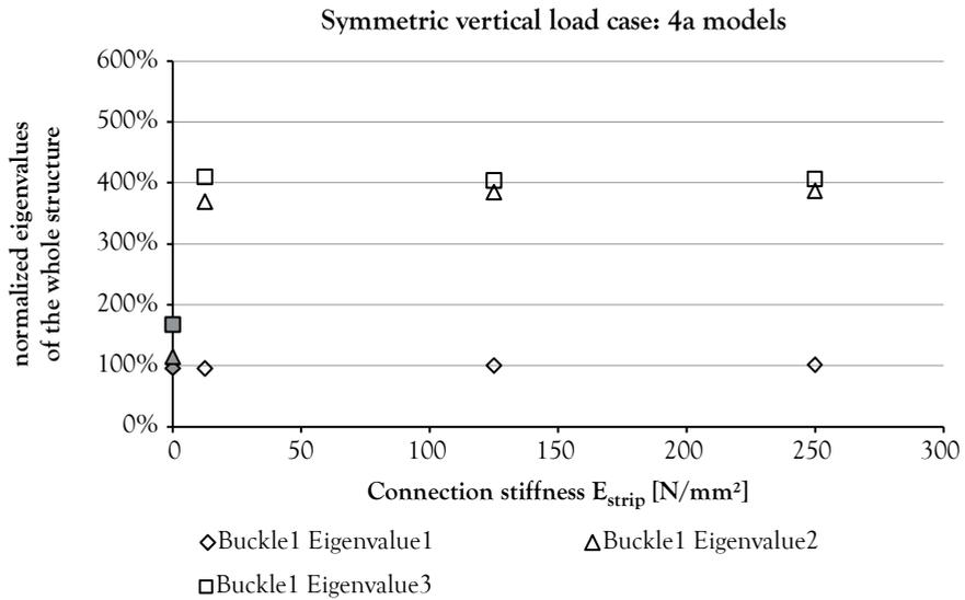
Figure 6-39: Influence of connection stiffness on absolute value of eigenvalues of the first buckle step for 4a models for the symmetric vertical load case (normalized for first eigenvalue in 4a\_putty model)
