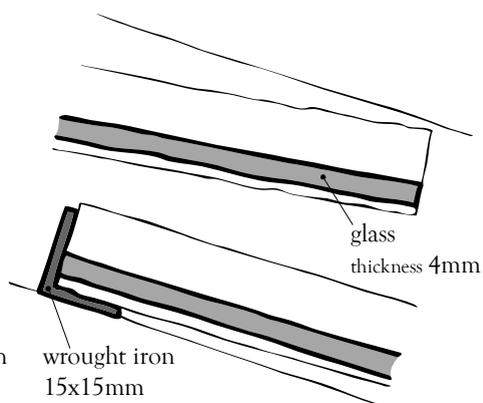
Figure 2-17: The longitudinal connection at the Saint-Hubertus Galleries: original detail before 1993-96 renovation campaign<sup>36</sup>
