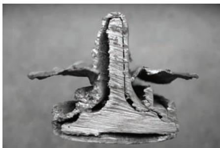
Figure 2-49: Picture of cross-section of glazing bar of outer roof of the double-walled roof (picture Origin, 2006-02-02)
