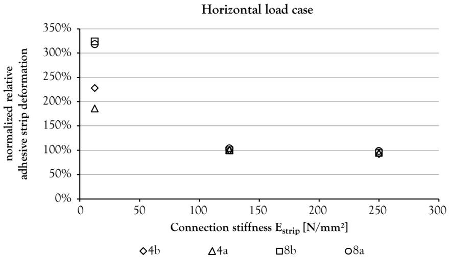
Figure 6-48: Relative deformation of the adhesive strips for the horizontal load case (normalized for 4a\_putty model)
