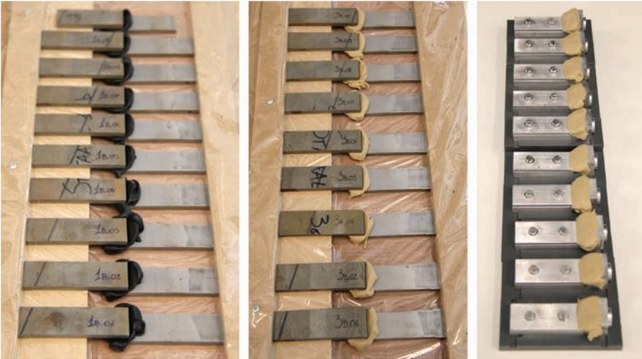
Figure 5-9: Sample series: (left) polymer sealant lap shear samples; (middle) putty sealant lap shear samples; (right) putty sealant compression samples
