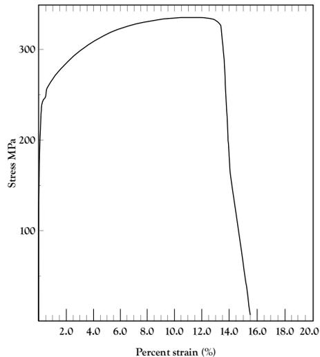
Figure 6-13: Stress-strain curve of iron material of Saint-Hubertus Galleries<sup>16</sup>
