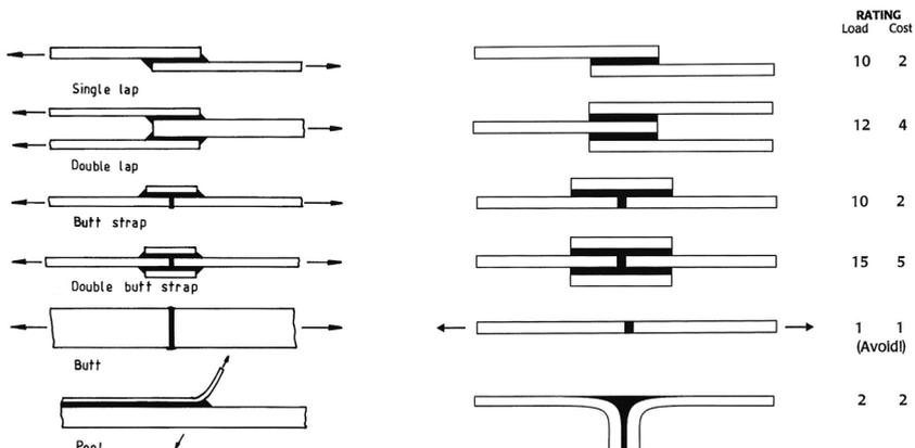
Figure 5-2: Comparison of common engineering adhesive joints and their structural efficiency based on strength and cost (the higher the load rating, the stronger is the joint)<sup>2</sup>
