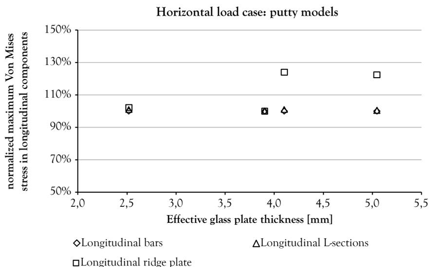
Figure 6-50: Influence of glass thickness on maximum Von Mises stress in the longitudinal iron components for putty models for the horizontal load case (normalized for 4a\_putty model)
