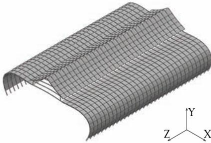
Figure 6-24: Deformed structure under symmetric vertical load (scale 50)
