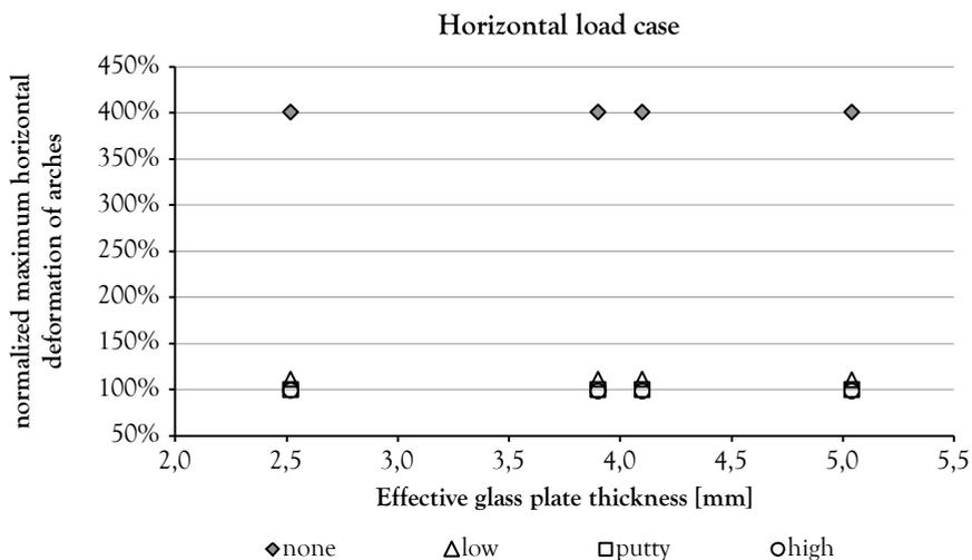
Figure 6-46: Maximum horizontal deformation of the arches for the horizontal load case (normalized for 4a\_putty model)
