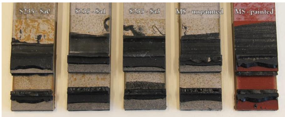
Figure 5-21: Adhesive failure of MS polymer adhesive sample series
