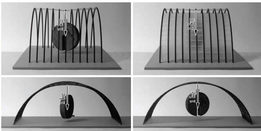
Figure 0-3: Dissipation of concentrated vertical weight in centre of the models:
