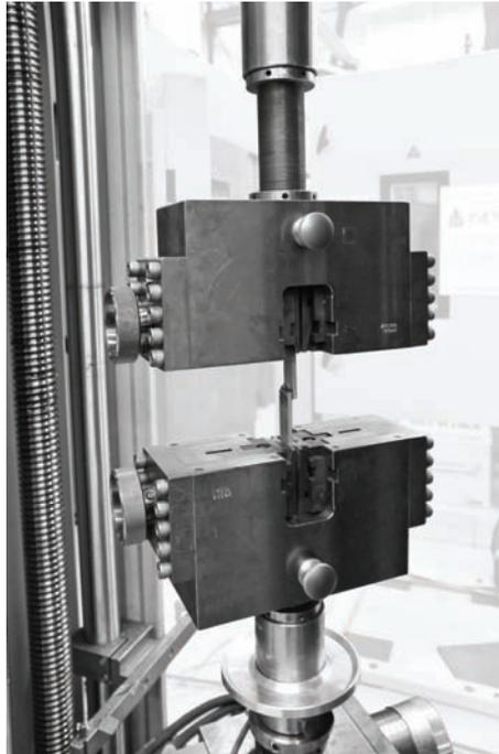
Figure 5-14: Single-lap shear tests at TU Delft with Zwick 250 kN universal electromechanical test machine
