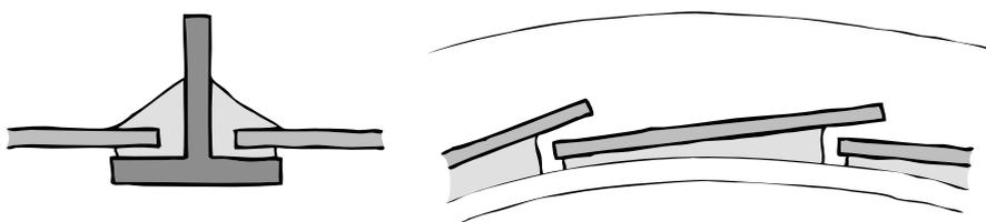
Figure 5-5: Filling capacity of sealant or adhesive: (left) typical 19th-century connection detail; (right) longitudinal connection of the same connection principle showing the difference in adhesive thickness alongside the length of the glass plate
