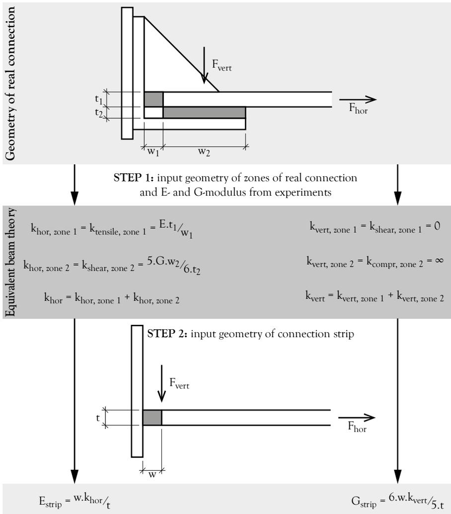
Figure 6-16: Scheme of calculation of fictitious material parameters
