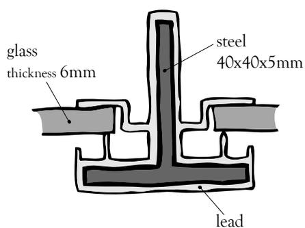
Figure 2-50: The construction techniques at the Institut des Arts et Métiers: detail as found in restoration report<sup>54</sup>
