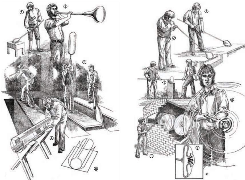
Figure 1-15: Production of cylinder glass<sup>78</sup> Figure 1-16: Production of crown glass<sup>79</sup>
