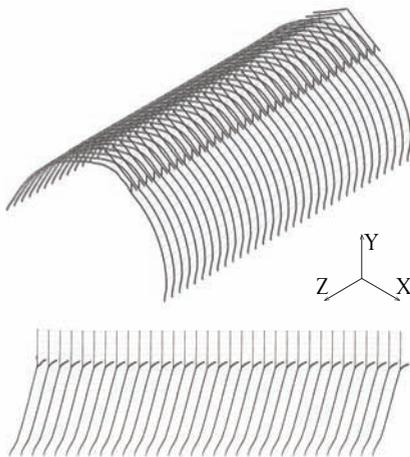
Figure 6-42: Deformed structure of 4a\_none model under horizontal load (scale 25)
