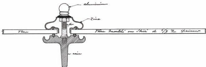
Figure 2-43: The patent glazing systems of the Ecole communale no. 10 "Karel Buls" (1902-06, Brussels, A. Samyn): detail as found on original plans<sup>50</sup>
