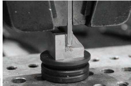
Figure 5-16: Avoiding eccentric forces by using a spherical cap hinge during compression tests
