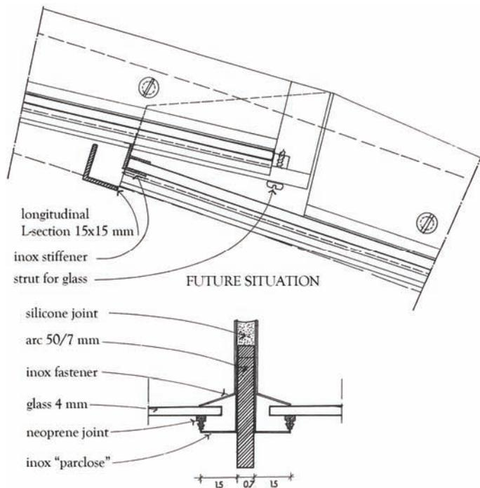
Figure 4-17: Transverse (bottom) and longitudinal (top) connection of Saint-Hubertus Galleries after 1993-97 restoration campaign<sup>86</sup>
