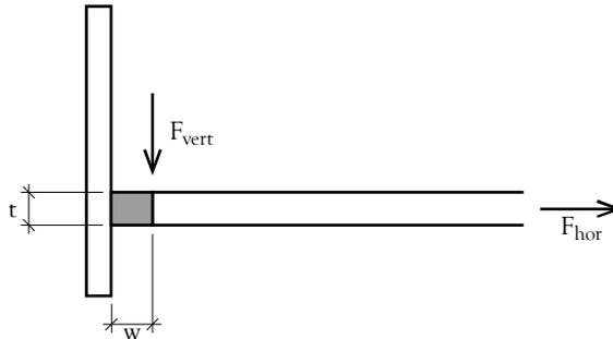
Figure 6-21: Geometric parameters of the connection strip
