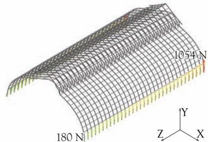
Figure 6-45: Vertical reaction forces at the bottom hinges for the 8a\_putty model under horizontal loading
