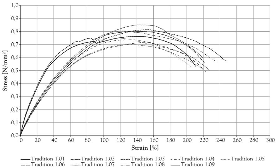
Figure 5-20: Stress-strain curve of polymer sealant single-lap shear tests
