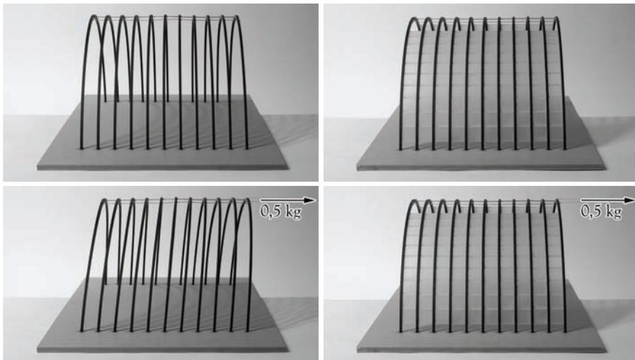
Figure 0-2: Stability of models loaded with horizontal weight:
