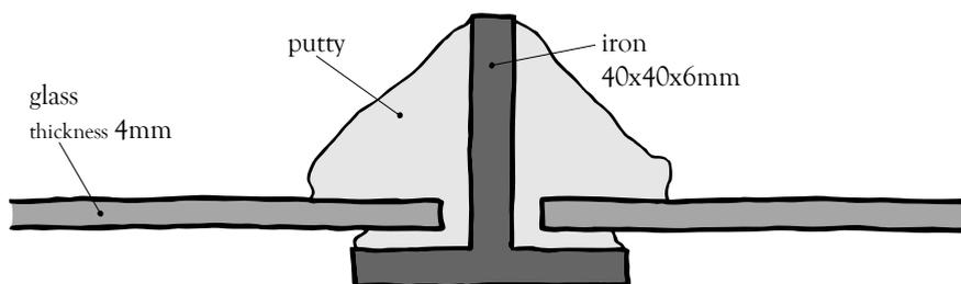
Figure 2-31: The transverse connection at the Winter Garden of the Royal Glasshouses of Laeken: detail as surveyed in present state
