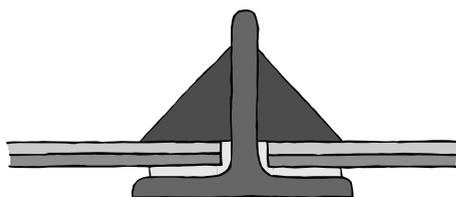
Figure 7-10: Interventions on standard T-shaped glazing bar: laminating historic glass (darker grey at bottom side) with new glass plates; replacing putty (partly or completely) by modern sealant or adhesive
