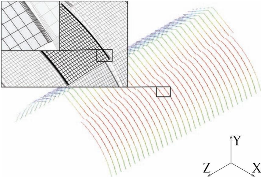
Figure 6-28: Deformation of adhesive material in Z-direction in the 4b\_low model under asymmetric perpendicular loading
