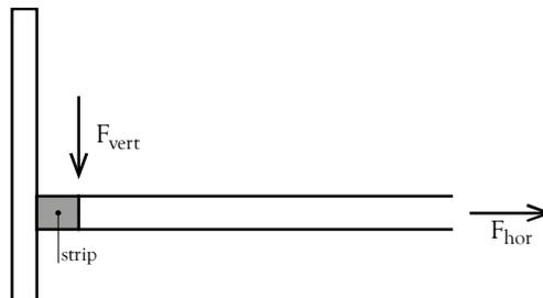
Figure 6-17: Loads on strip of fictitious material that simulates the connection stiffness
