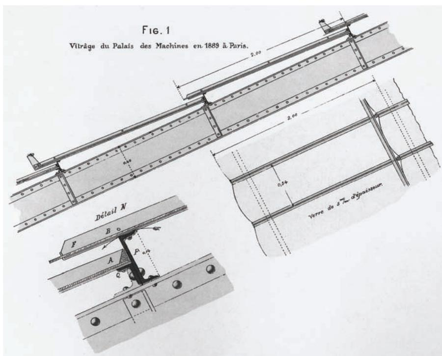
Figure 2-12: Glazing of Galeries des Machines, Paris, 1889<sup>26</sup>
