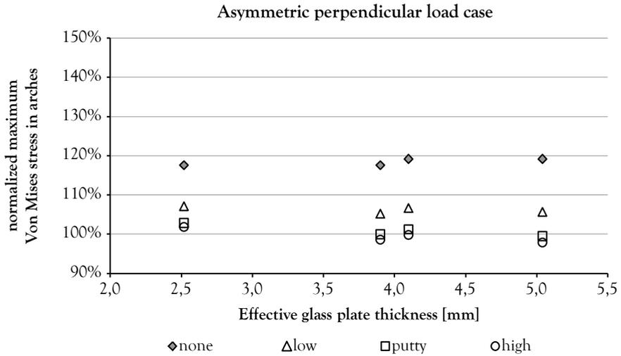
Figure 6-35: Maximum Von Mises stress in the arches for the asymmetric perpendicular load case (normalized for 4a\_putty model)
