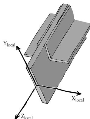
Figure 6-9: Glazing bars connected to iron arch
