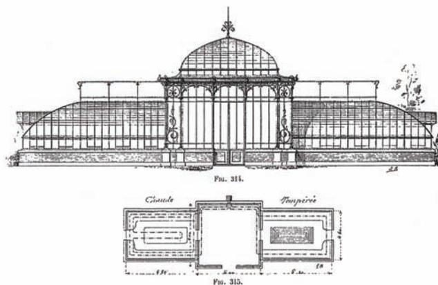
Figure 2-3: Description of iron and glass construction: example of a wintergarden construction (façade and plan)<sup>9</sup>
