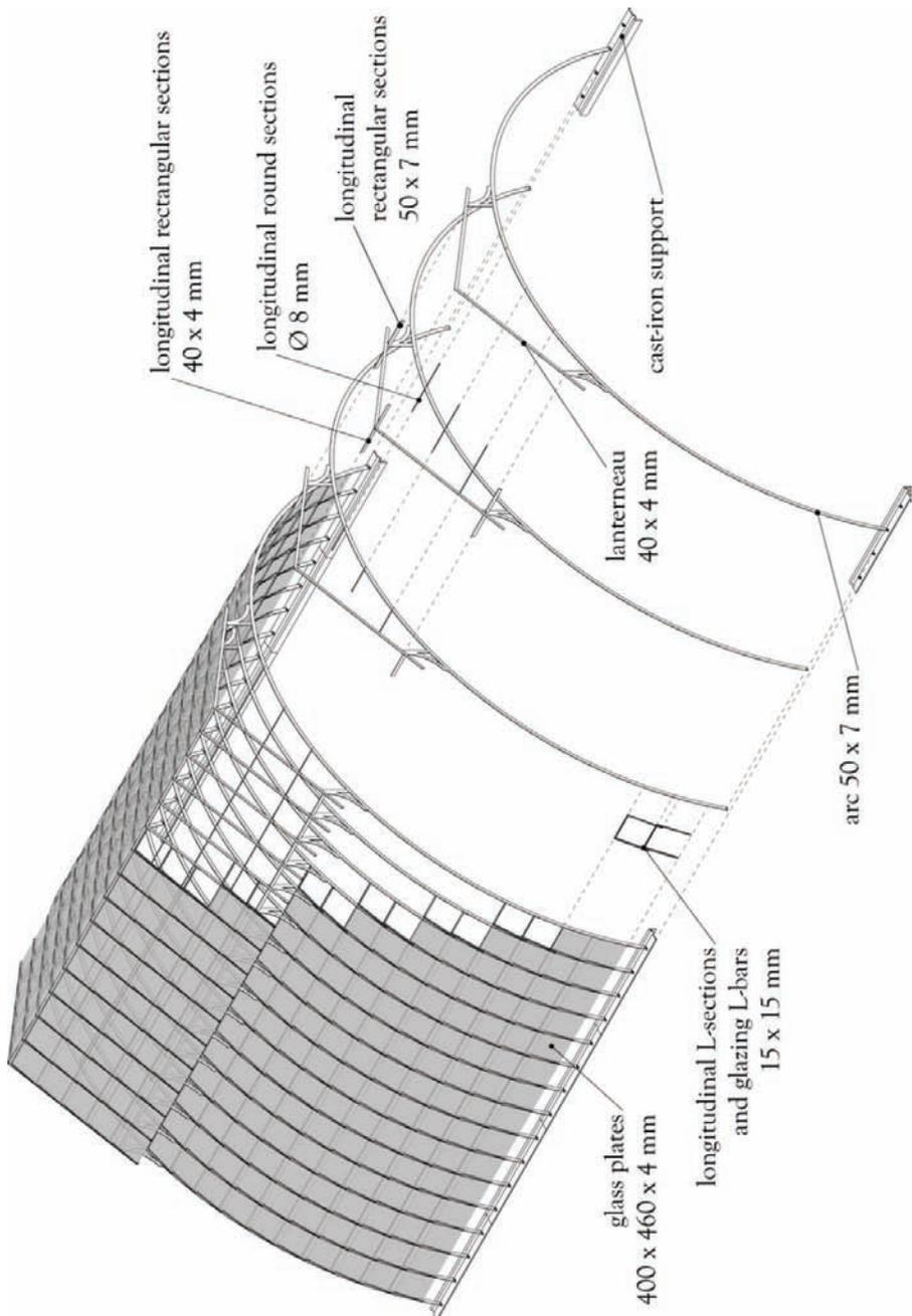
Figure 4-13: Isometric exploded view of iron and glass roof of Saint-Hubertus Galleries<sup>68</sup>
