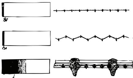
Figure 2-1: Study of different glazing bar systems and the light they admit: (left) ground surface of glasshouse with shaded area, (right) compared glazing systems (iron curvilinear, iron ridge-and-furrow, and wooden glazing bars)<sup>2</sup>
