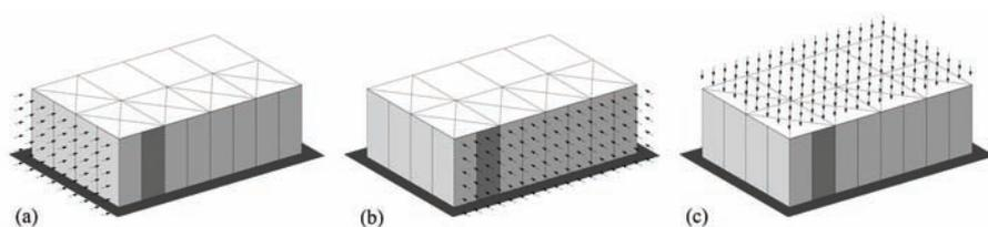
Figure 3-1: Actions on individual glass panel (dark grey panel): (a) in-plane shear force due to wind force in longitudinal direction; (b) out-of-plane bending due to wind force in transversal direction; (c) in-plane compressive force due to gravity loads on roof<sup>7</sup>
