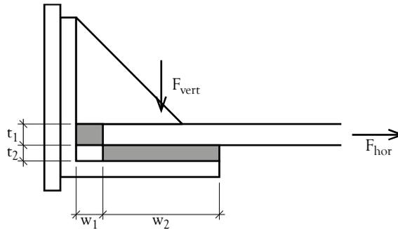
Figure 6-20: Geometric parameters of the two loaded zones on the real connection detail
