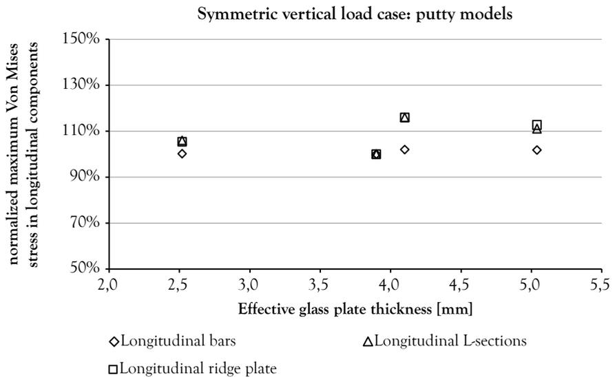
Figure 6-38: Influence of glass thickness on maximum Von Mises stress in the longitudinal iron components for putty models for the symmetric vertical load case (normalized for 4a\_putty model)
