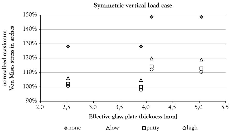
Figure 6-36: Maximum Von Mises stress in the arches for the symmetric vertical load case (normalized for 4a\_putty model)
