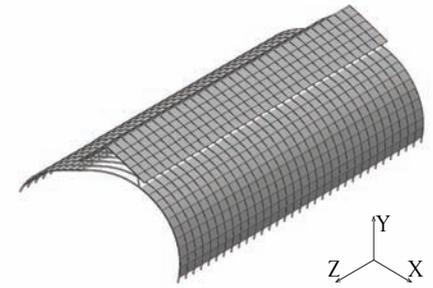
Figure 6-25: Deformed structure under asymmetric vertical load (scale 10)
