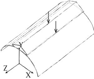
Figure 6-10: Concentrated maintenance load
