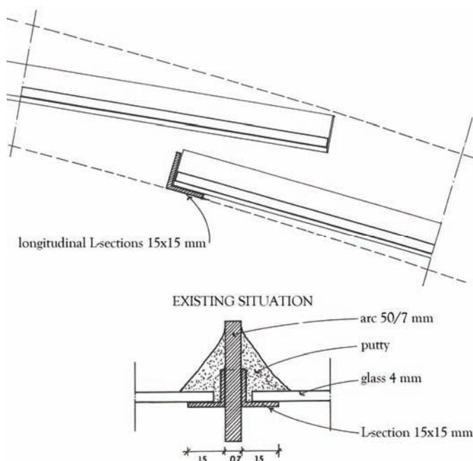
Figure 4-16: Transverse (\*) (bottom) and longitudinal (top) connection of Saint-Hubertus Galleries before 1993-97 restoration campaign<sup>83</sup>
