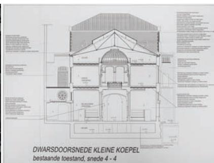
Figure 4-26: Transversal section through small roof light<sup>88</sup>
