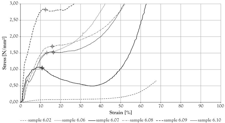
Figure 5-18: Stress-strain curves of putty sealant compression tests after 3 months curing
