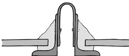
Figure 2-10: Transverse connection: dilatation joint with copper strips
