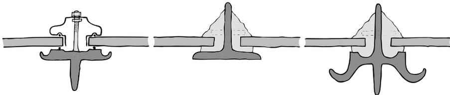
Figure 5-1: Transverse connection in glass roofs: section system with rubber strips (left); simple T-section with putty (middle); and moulded T-section with gutters sealed with putty (right)
