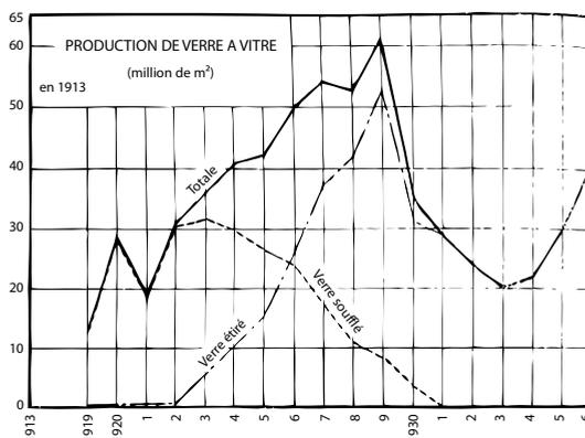
Figure 1-24: Gradual switch from blown to drawn glass<sup>214</sup>
