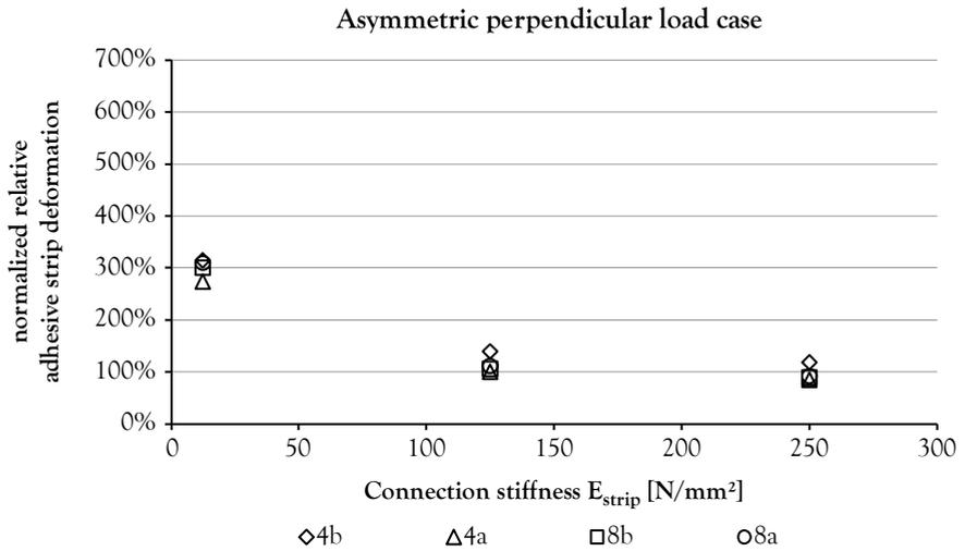
Figure 6-33: Relative deformation of the adhesive strips for the asymmetric perpendicular load case (normalized for 4a\_putty model)
