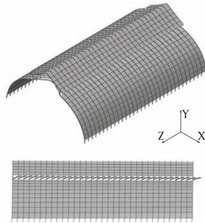
Figure 6-43: Deformed structure of 4a\_putty model under horizontal load (scale 25)
