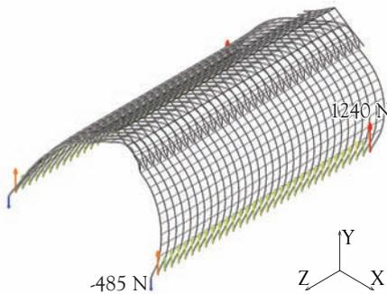
Figure 6-44: Vertical reaction force at the bottom hinges for the 8a\_none model under horizontal loading
