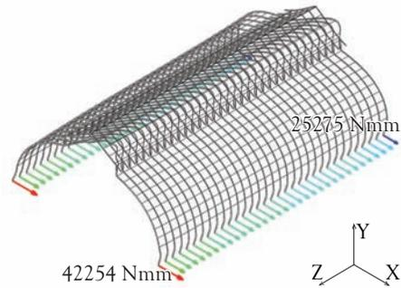
Figure 6-41: Reaction moments at the bottom hinges for the 4b\_low model under horizontal loading
