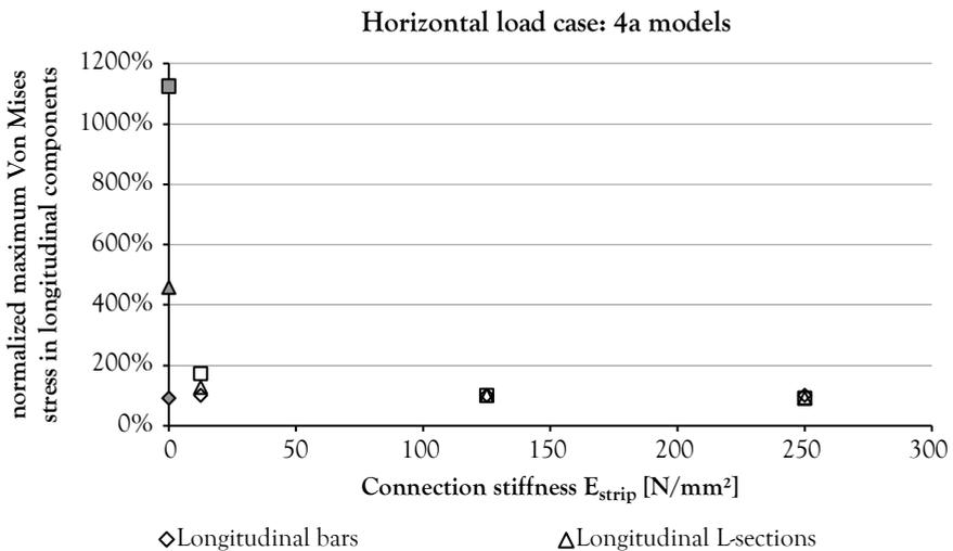
Figure 6-49: Influence of connection stiffness on maximum Von Mises stress in the longitudinal iron components for 4a models for the horizontal load case (normalized for 4a\_putty model)
