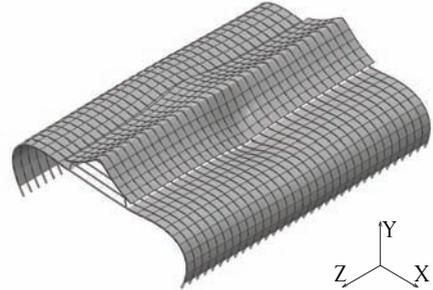
Figure 6-23: Deformed structure under asymmetric concentrated load (scale 150)
