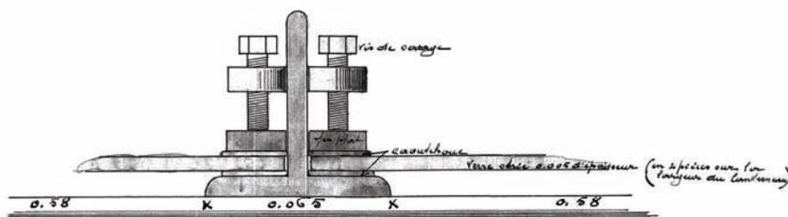
Figure 2-44: The patent glazing systems of the Ecole communale no. 7 "Baron Steens" (1896-97, Brussels, A. Samyn): detail as found on original plans<sup>51</sup>
