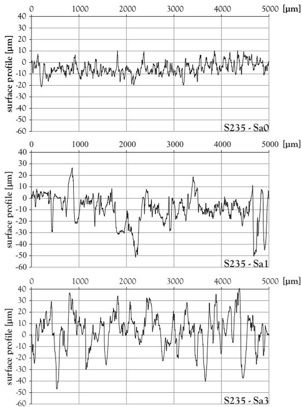
Figure 5-23: Surface profiles of series S235 – Sa0 (top), series S235 – Sa1 (middle) and series S235 – Sa3 (bottom)
