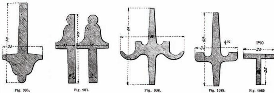
Figure 2-7: Sections of iron glazing bars mentioned in manuals and course books: example of elaborate drawings<sup>19</sup>
