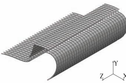
Figure 6-27: Deformed structure under asymmetric perpendicular load (scale 10)
