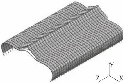
Figure 6-26: Deformed structure under symmetric perpendicular load (scale 150)
