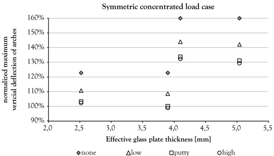
Figure 6-32: Maximum deflection of the arches for the symmetric concentrated load case (normalized for 4a\_putty model)
