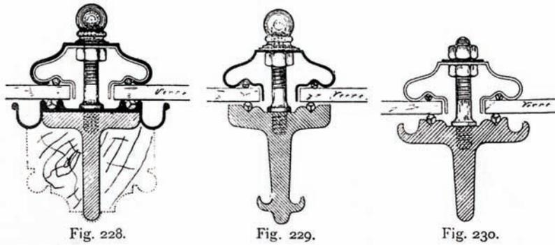
Figure 2-6: Sections of iron glazing bars mentioned in manuals and course books: example of patent glazing systems<sup>18</sup>
