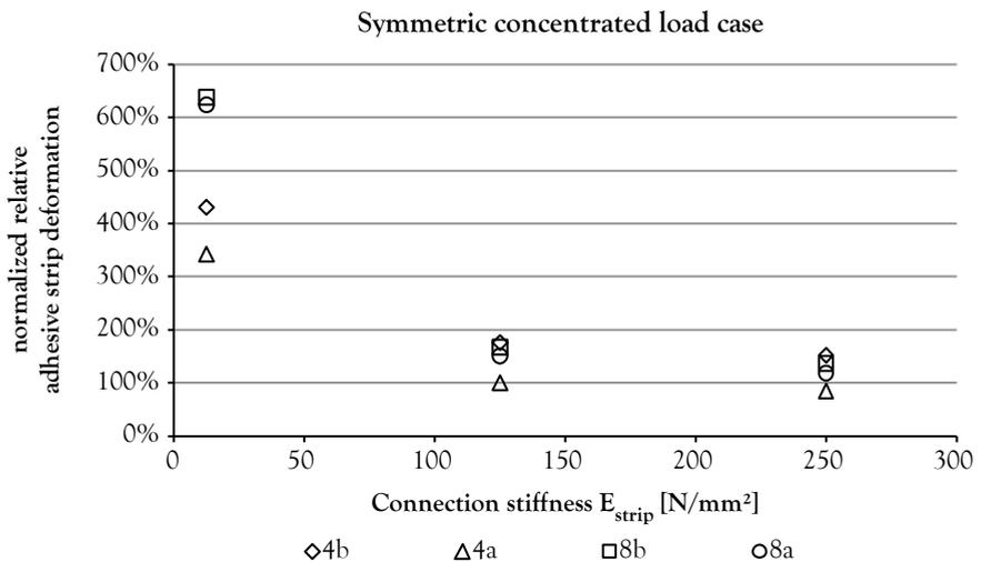
Figure 6-34: Relative deformation of the adhesive strips for the symmetric concentrated load case (normalized for 4a\_putty model)
