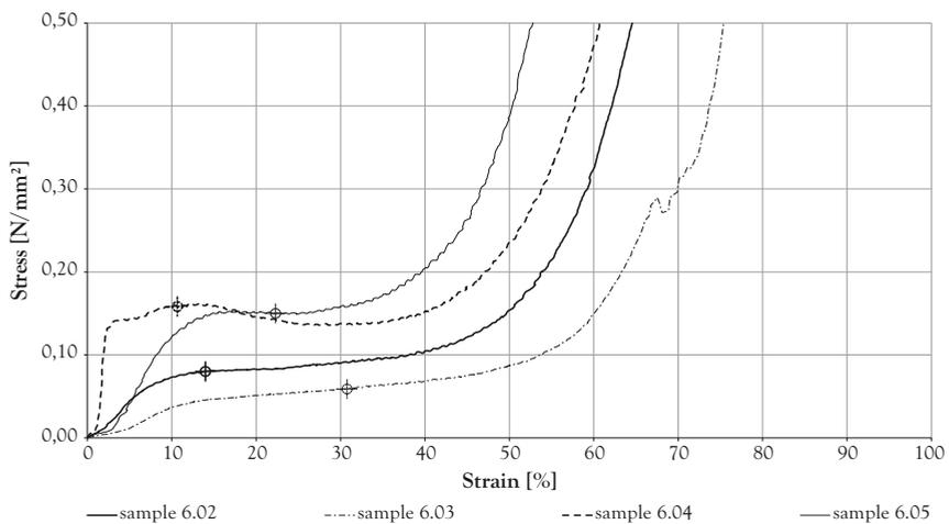
Figure 5-17: Stress-strain curves of putty sealant compression tests after 1 month curing
