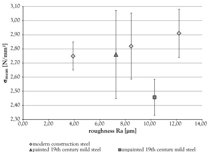
Figure 5-24: Roughness influence graph on modern construction steel and 19th century unpainted mild steel
