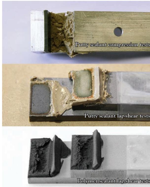
Figure 5-19: Failure surfaces: (top) putty sealant compression tests; (middle) adhesive failure of putty sealant lap shear test; (bottom) cohesive failure of polymer sealant lap shear tests
