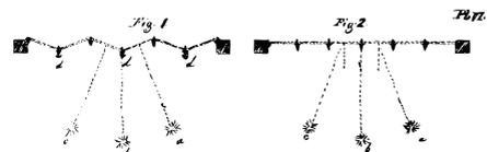
Figure 2-2: Study of roof geometry (ridge-and-furrow and flat roof) to improve the admission of light<sup>3</sup>
