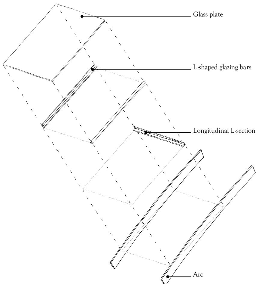
Figure 6-2: Exploded view of placing glass covering of the Saint-Hubertus Galleries
