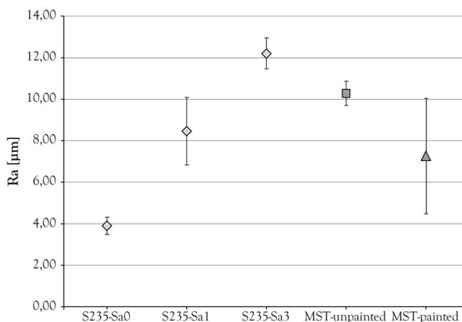
Figure 5-13: Roughness measurements on MS polymer adhesive sample sets
