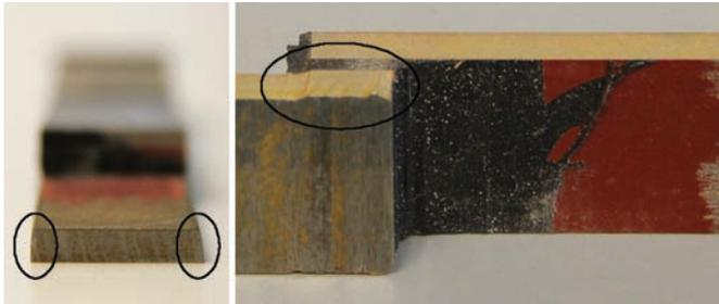
Figure 5-11: Geometrical imperfections due to water jet cutting: (left) tapered cross-section; (right) deformed cut line
