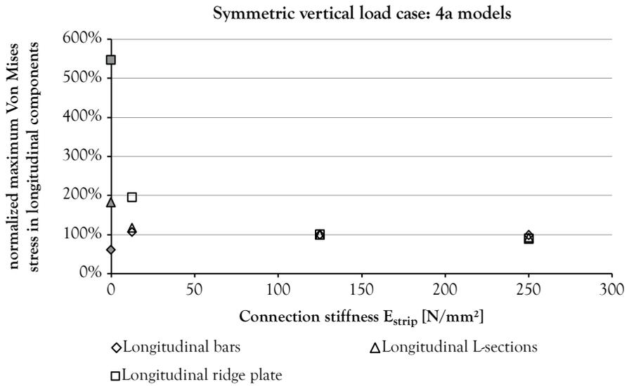
Figure 6-37: Influence of connection stiffness on maximum Von Mises stress in the longitudinal iron components for 4a models for the symmetric vertical load case (normalized for 4a\_putty model)
