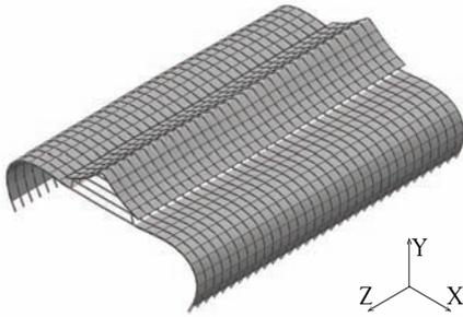
Figure 6-22: Deformed structure under symmetric concentrated load (scale 150)
