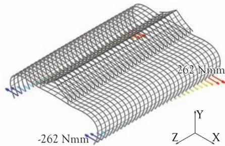
Figure 6-29: Reaction moments at the bottom hinges (about X-axis) for the 4b\_low model under symmetric vertical loading
