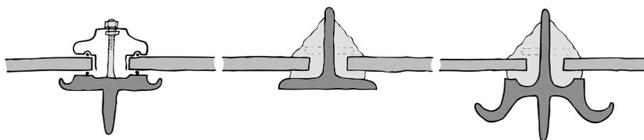
Figure 2-9: Transverse connection in glass roofs: section system with rubber strips (left); simple T-section with putty (middle); and moulded T-section with gutters sealed with putty (right)
