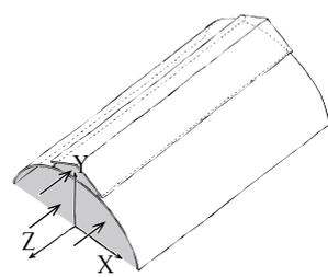
Figure 6-12: Horizontal wind load
