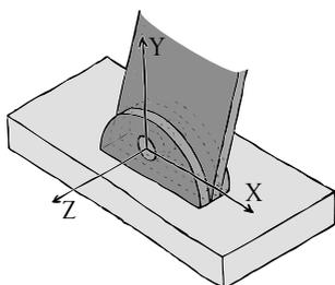
Figure 6-7: Hinged connection at bottom of iron arches
