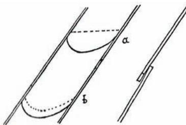
Figure 2-13: Cutting patterns for bottom edge of glass plates to keep rain away from putty connection<sup>27</sup>
