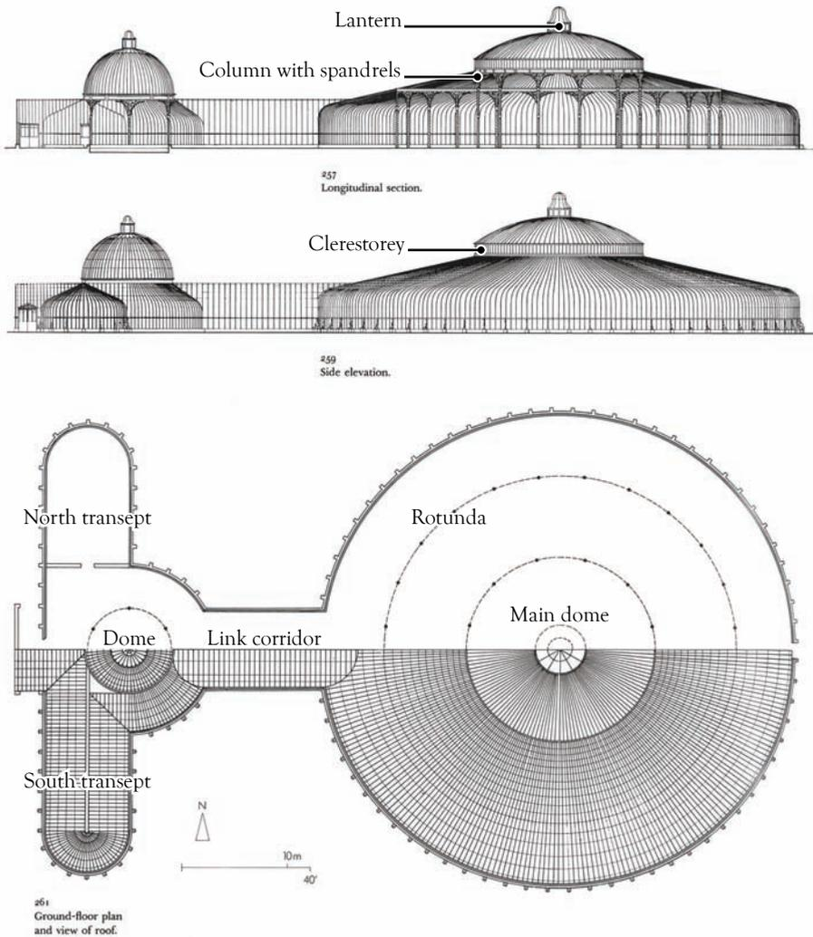
Figure 4-2: Ground plan, section and elevation of Kibble Palace<sup>19</sup>
