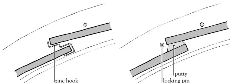
Figure 2-11: Zinc hook (left) or putty and a locking pin (right) for the longitudinal connection
