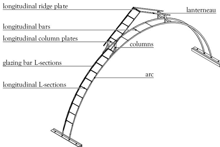
Figure 6-3: One segment of the Saint-Hubertus Galleries without glass plates with the nomenclature of the iron sections for this chapter
