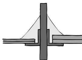
Figure 7-11: Different proportions of glass plate thicknesses compared to the iron glazing bars when applying laminated glass in historic connection detail: (left) 2 panes of 2 mm thickness; (right) 2 panes of 4 mm thickness
