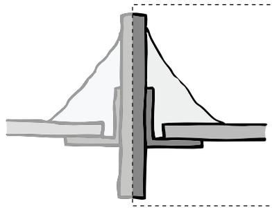
Figure 6-14: Connection detail at Saint-Hubertus Galleries with annotation of half of the connection that will be illustrated in following figures
