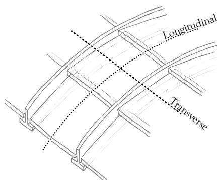
Figure 2-5: Transverse and longitudinal connection in a glass roof
