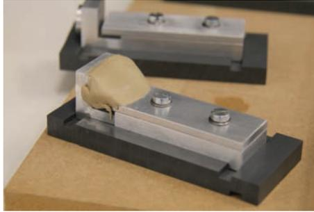
Figure 5-8: Mould for the manufacture of the putty compression samples
