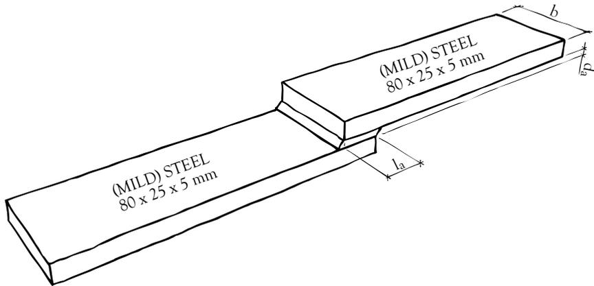
Figure 5-10: Specimen geometry of the lap shear samples in steel or mild steel
