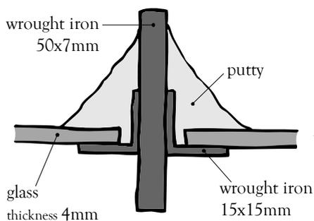
Figure 2-16: The transverse connection at the Saint-Hubertus Galleries: original detail before 1993-96 renovation campaign<sup>35</sup>
