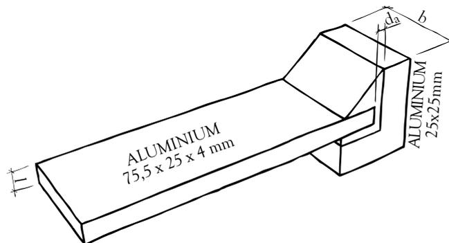
Figure 5-7: Specimen geometry of the putty sealant compression samples in aluminium
