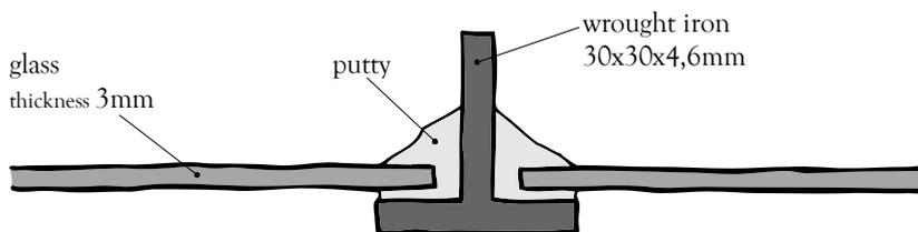
Figure 2-24: The transverse connection at the Victoria Regia Glasshouse: detail as surveyed in present state
