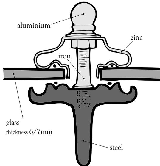
Figure 2-42: The transverse connection at the Ecole communale no. 10 "Karel Buls": detail as found on plan
