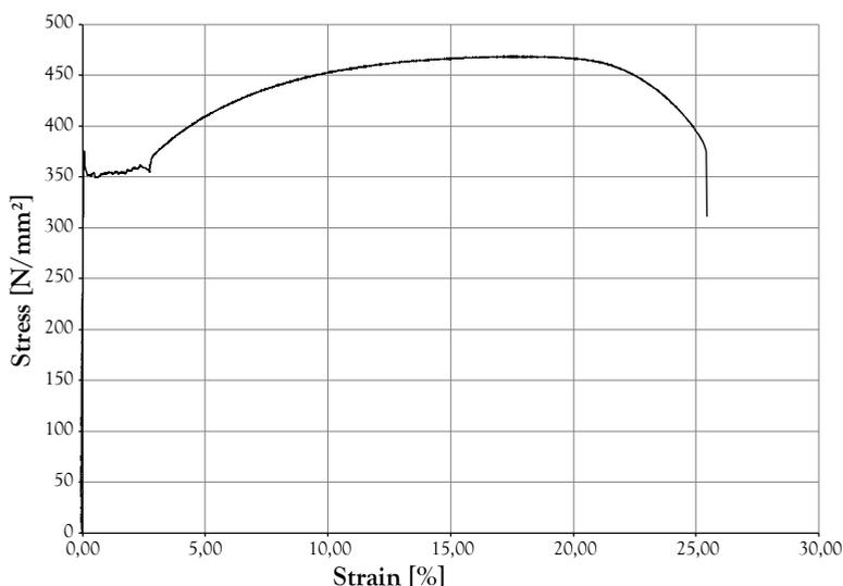
Figure 5-4: Stress-strain curve of the mild steel substrates from the Janlet wing of the Museum of Natural Sciences in Brussels<sup>15</sup>
