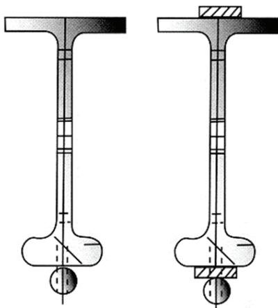
Figure 7-14: Palm House at Kew Gardens: adding sections to original cross-section to strengthen the wrought-iron arches during the 1985-88 restoration campaign<sup>13</sup>
