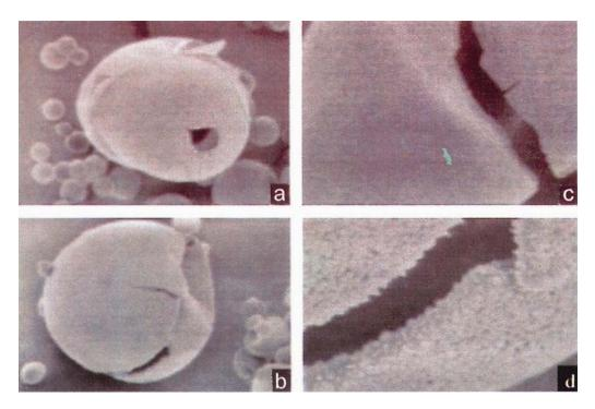
Fig. 3—Scanning electron microscopy surface images of spherical porous Trojan particle. [Scale bars: 10 µm a, b and 2 µm c,d]
