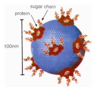
Fig 4—Schematic presentation of Smart Particle (nanoparticles with targeting moieties attached on the surface)
