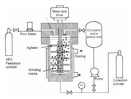
Fig 1—Schematic of the High Pressure Media Mill (HPMM)
