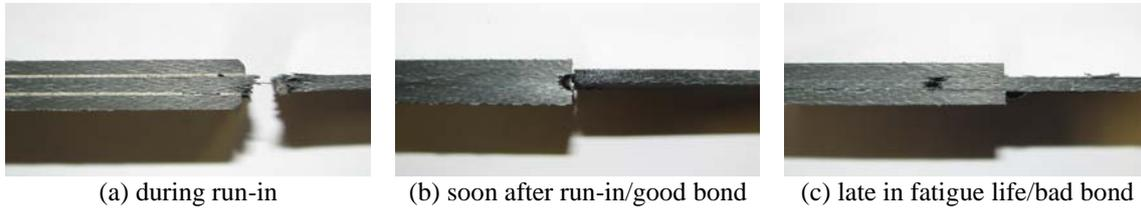
**Figure 3** Overview of the occurring tab failures during fatigue experiments
