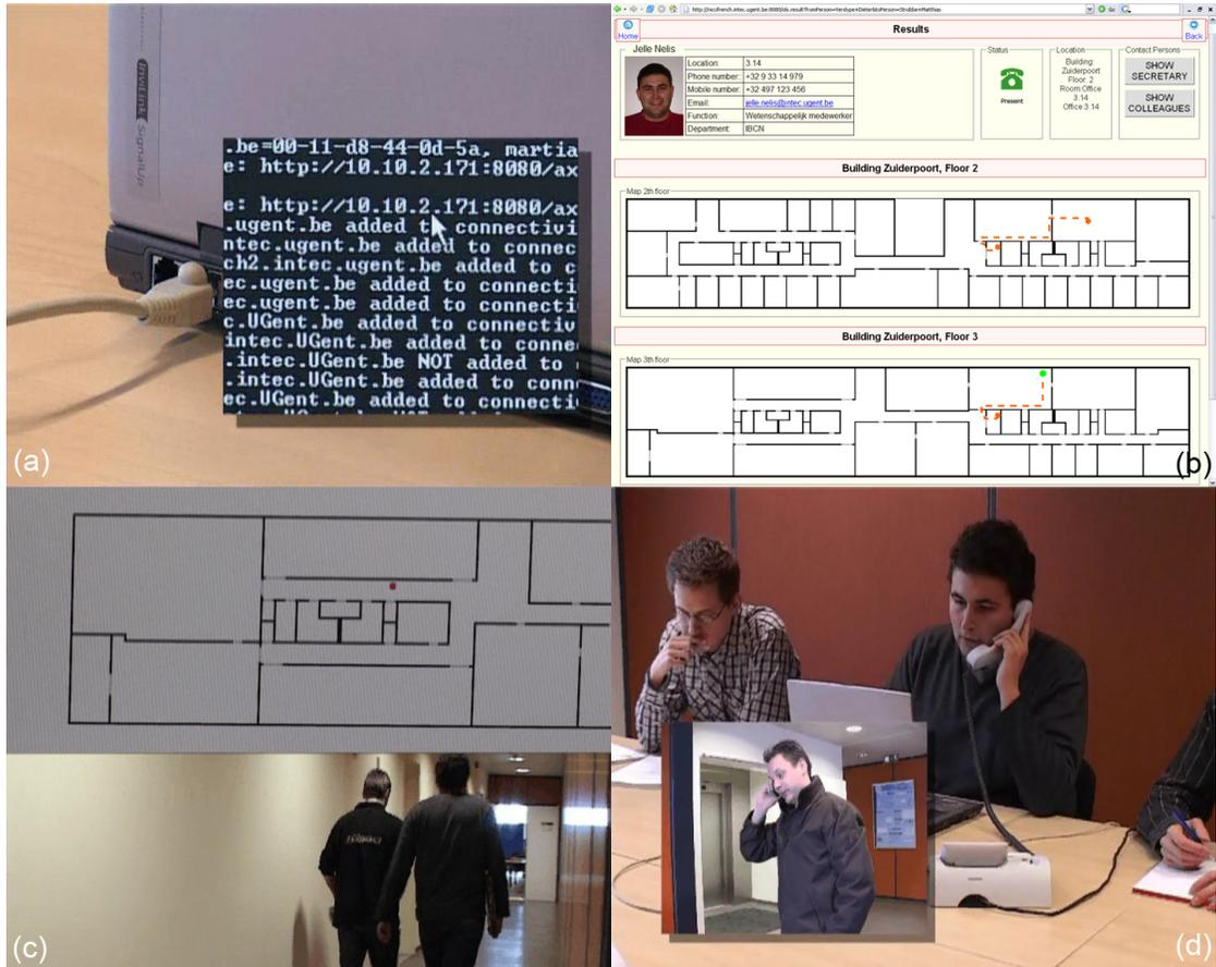
Fig. 3. Desk sharing office use case. (a) SNMP based localization: a laptop plugged into the company network is detected and localized. (b) Screenshot of the web application. (c) WiFi based localization: walking employee is tracked. (d) By clicking on the telephone icon, an automatic call is set up between visitor and employee.
