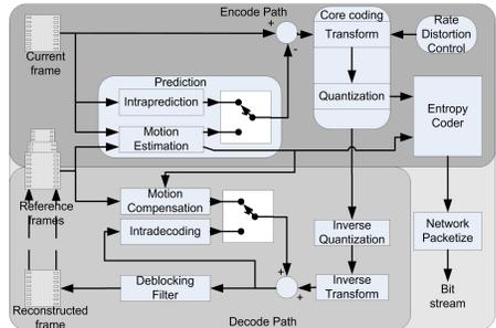
Figure 1. H.264 encoder and decoder top-level
