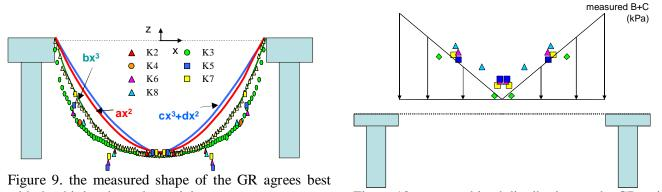
with the third-order-polynomial Figure 10. measured load distribution on the GR strip
