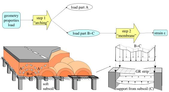
Figure 1. In most design methods, the calculation of the GR strain due to vertical load is carried out in two steps.
