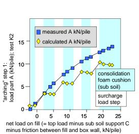
Figure 6. Measured and calculated (CUR/EBGEO) result of step 1 (arching)
