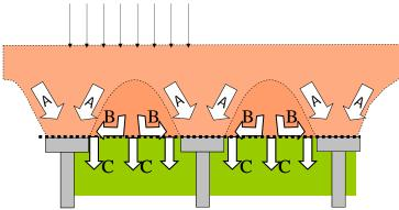
Figure 2. Load distribution in a piled embankment.
