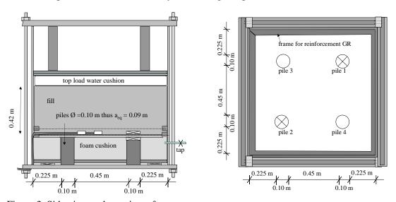
Figure 3. Side view and top view of test set-up
