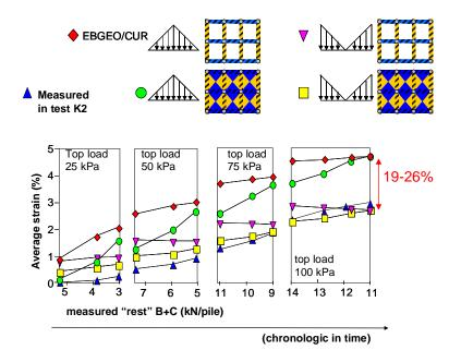
Figure 11. Comparison measurements and calculations step 2, effect of modifications CUR/EBGEO calculation model: a. modification load distribution (from triangular shape to inverse triangular shape) and b. modification subsoil support (from below GR strip only to below entire, diamond shaped GR area)
