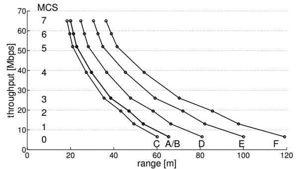
Fig. 3. Physical throughput versus calculated range for 802.11n reference receiver, SISO, frequency 2.4 GHz, bandwidth 20 MHz, all types of environment (A - F). The calculation is based on the TGn channel model.
