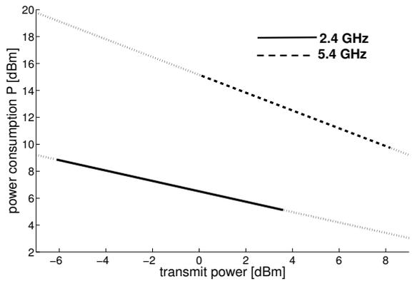
Fig. 6. Required total power consumption (due to radiation) vs transmit power, calculated based on PL model, proposed for large conference rooms. The dotted line indicates that the range is out of the region where the PL model could be experimentally determined.
