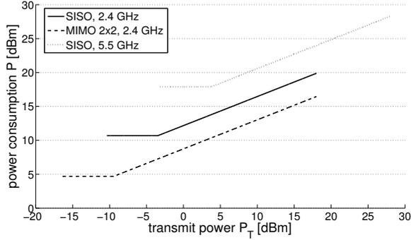
Fig. 5. Required total power consumption (due to radiation) vs transmit power, calculated based on TGN channel model.
