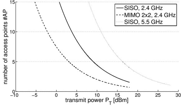
Fig. 4. Required number of access points vs transmit power, calculated based on TGN channel model.
