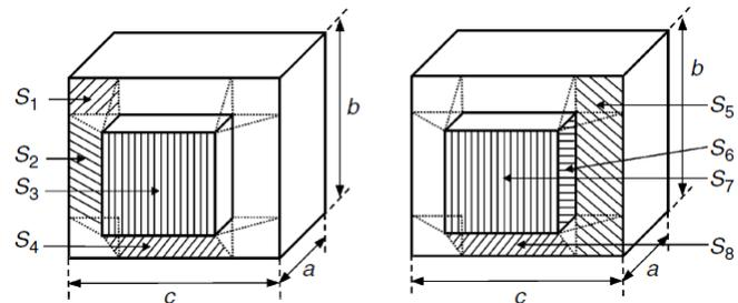
Fig. 1. The equivalent surfaces of an EE core transformer:
