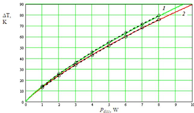
Fig.5 Temperature rise  $\Delta T$  as function of the dissipated power  $P_{diss}$  for enameled (1) and black painted (2) surfaces, box 42x42x15mm, horizontal orientation,  $T_a=25^\circ C$ . solid curves: model results; dash lines: experimental results.
