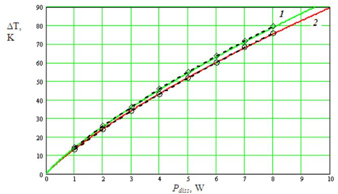
Fig.6 Temperature rise  $\Delta T$  as function of the dissipated power  $P_{diss}$  for enameled (1) and black painted (2) surfaces, box 42x42x15mm, vertical orientation,  $T_a=25^\circ C$ . solid curves: model results; dash lines: experimental results.
