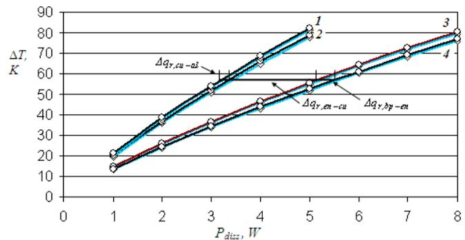
Fig.4 Temperature rise  $\Delta T$  as function of the dissipated power  $P_{diss}$  for different surfaces, box 42x42x15mm, bold curves: horizontal orientation of the model; light curves: vertical orientation of the model. (note that the light curves are just below the bold curves) 1: bright aluminium; 2: unpolished copper; 3: enamelled copper 4: black painted copper.
