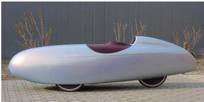
Fig. 4: Mango "quest" human powered vehicle type "velomobiel" (Wq) [5]
