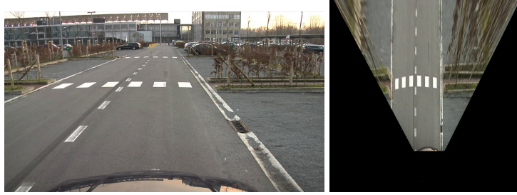
Fig. 1. Example of a test frame (left), and its ground plane backprojection (right).
