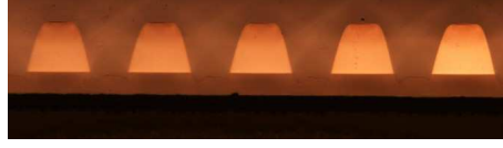
Figure 4. Polished end-facet cross-section of an array of laser ablated 50 \times 50\text{-}\mu\text{m}^2 waveguides, on a pitch of 125\text{-}\mu\text{m} .
