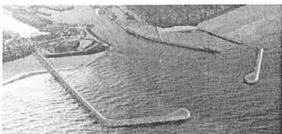
Figure 1 - New harbour access with two new breakwaters
