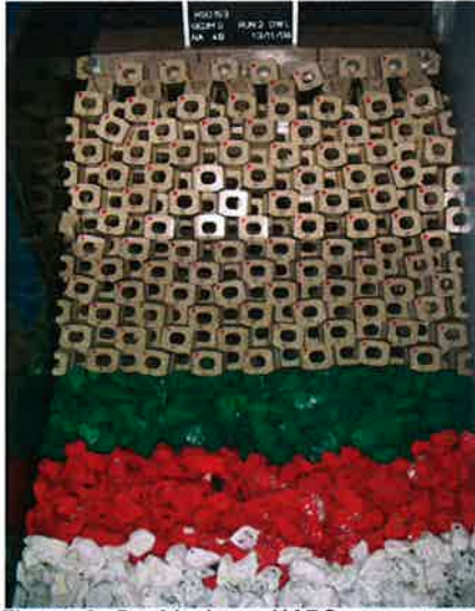
Figure 6. Double layer HAROs as armour layer on the seaside of the breakwaters
