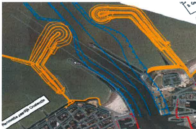
Figure 1. Old harbour entrance (grey lines) is replaced by the new entrance (blue lines) and protected by 2 new breakwaters (yellow lines).
