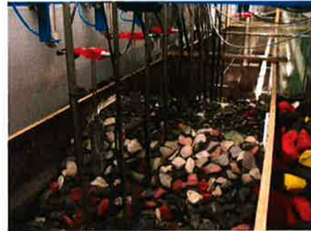
Figure 6 : Wave gauges in perforated tubes (stage 2)
