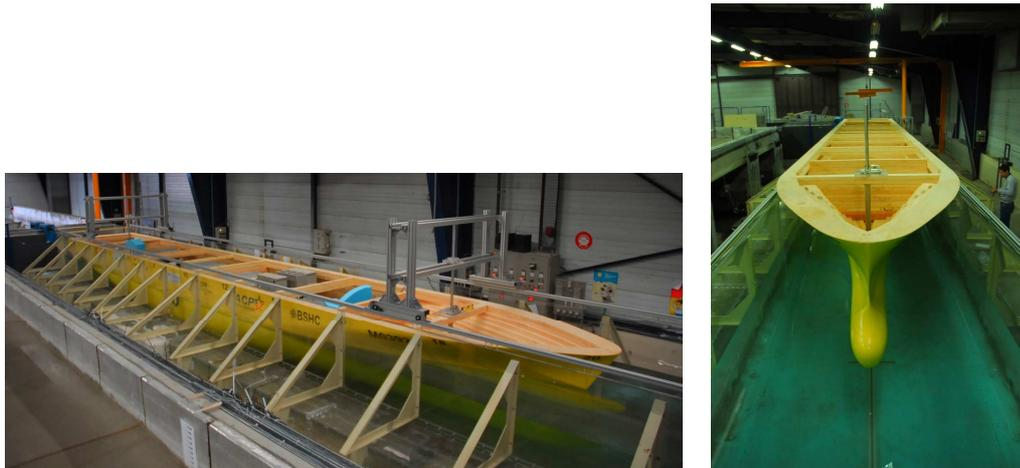
**Figure 5: View of the Post-Panamax container ship model**
