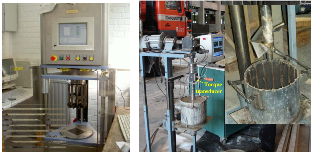
Figure 2. Left: ConTec Viscometer. Right: Tattersall Mk-II rheometer.
