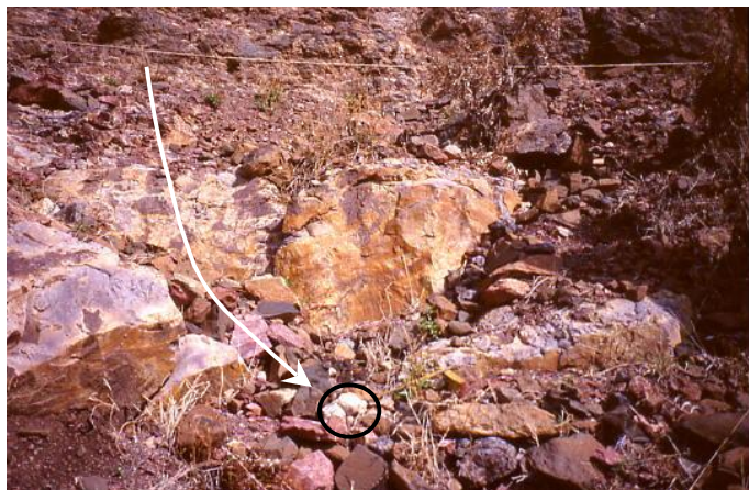
Fig. 5. Tracers (white limestone) displaced over a distance of 6 m in 20 months (Harena rangeland, March 2001). The horizontal rope at the back witnesses original tracer position.
