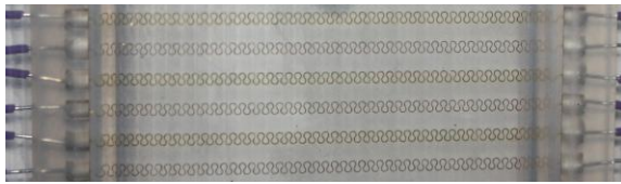
Figure 5: Horseshoe-shaped interconnections embedded into PDMS.
