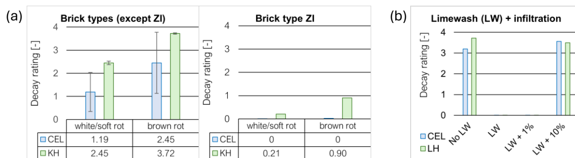
Figure 8. Simulation results of the decay rating on a 4-year period per parameter: (a) average values for the 7 simulated brick types except ZI (left) and results for brick type ZI (right), (b) results for limewash with different infiltration rates (%). Values are displayed for both CEL and LH insulation.
