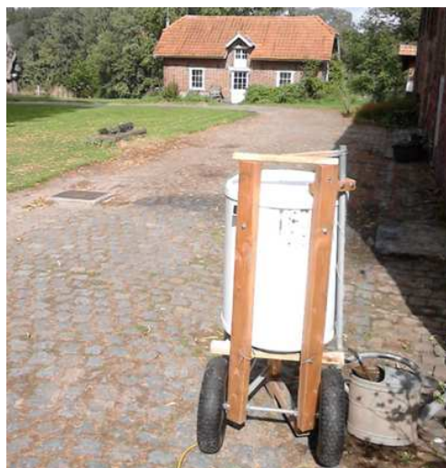
Fig. 4: A dump resistor for weed killing
