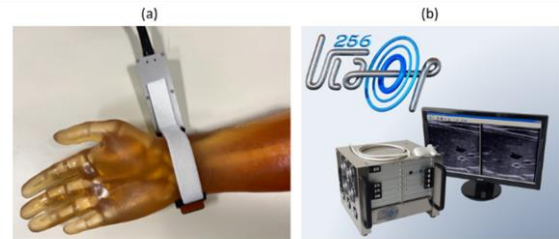
Fig. 1. Setup for the experiment a) Array attached to arm phantom with Velcro band b) Ultrasound scanning system (ULA-OP 256)
