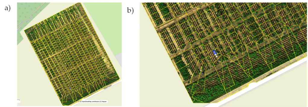
Figure 11. Orthomosaic (a) full field; (b) detail) of a flight generated with a flight overlap of 80% in horizontal and vertical direction. The yellow lines indicate the area taken from each single image. Notice the constant pattern in the core of the images, whereas the edges typically have larger areas from a single image, increasing the risk of anisotropic effects. Image taken from Agisoft Metashape from a dataset of multispectral imagery (MicaSense RedEdge-MX Dual), acquired on 07/10/2024, over a potato field in Bottelare, Belgium (lat: 50.9612°N, lon: 3.7677°E), at a flight height of 32 m.
