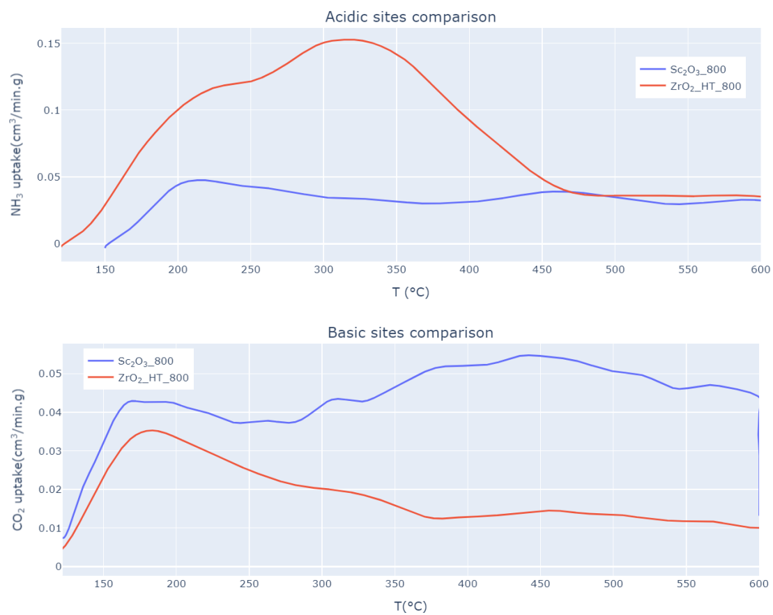
Figure 2: NH 3 -TPD (top) and CO 2 -TPD (bottom) for ZrO 2 _HT_800 and Sc 2 O 3 _800 catalyst samples.
