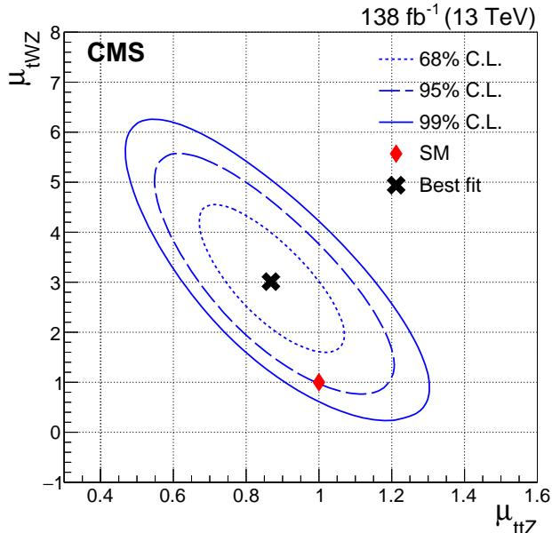
Figure 4: Two-dimensional likelihood scan of the signal strengths of tWZ ( $\mu_{\text{tWZ}}$ ) vs.  $\text{t}\bar{\text{t}}\text{Z}$  ( $\mu_{\text{ttZ}}$ ). The blue lines show the 68%, 95%, and 99% confidence level contours. The black cross represents the best-fit value, while the red diamond the SM expectation.
