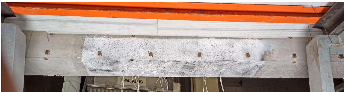
214 Figure 5. The compressed side of the beams monitored using the Digital Image Correlation (DIC).
