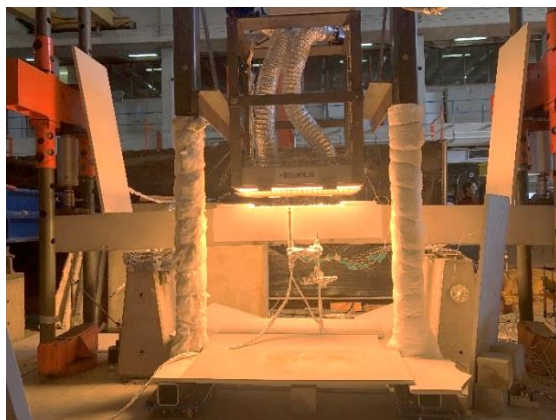
Figure 7: Reinforced concrete beam in reversed 4-point bending setup with the middle part exposed to fire using the electric radiant panel.
