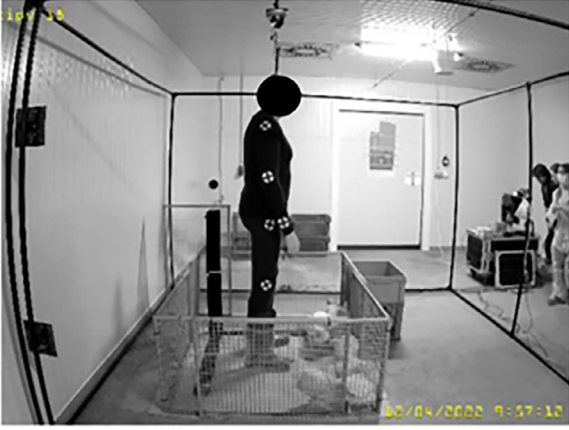
Figure 2. Setting of markers placed on the body of the test person to identify the different body parts for analysis.
