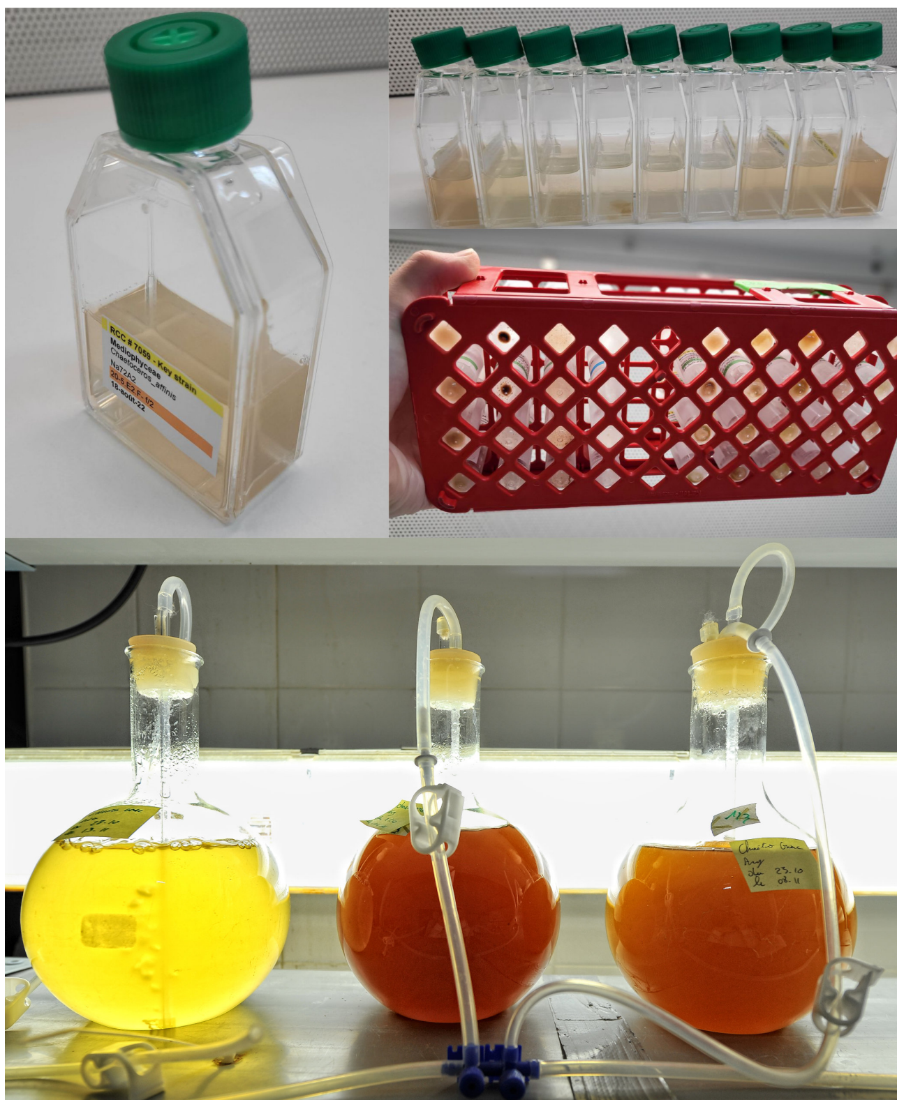
Figure 8: Cultures of diatoms at the Roscoff Culture Collection using either small culture flasks, tubes or larger glass containers with a bubbling system.
