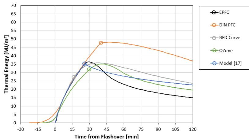
Figure 5. Total in-depth accumulated thermal energy within the analysed structural element according to different methods, highlighting the instant of maximum fire temperature (circles).
