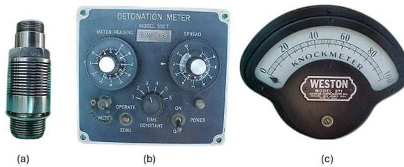
Figure 2.7: The D1 pressure pickup (a) - detonation meter (b) - knockmeter (c).
