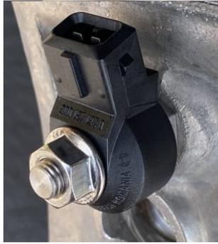
*Figure 4.5: A production engine knock sensor, mounted on the engine block.*
