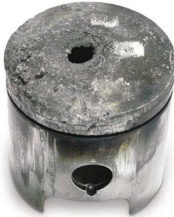
*Figure 2.5: A damaged piston, the result of extensive exposure to engine knock.*
