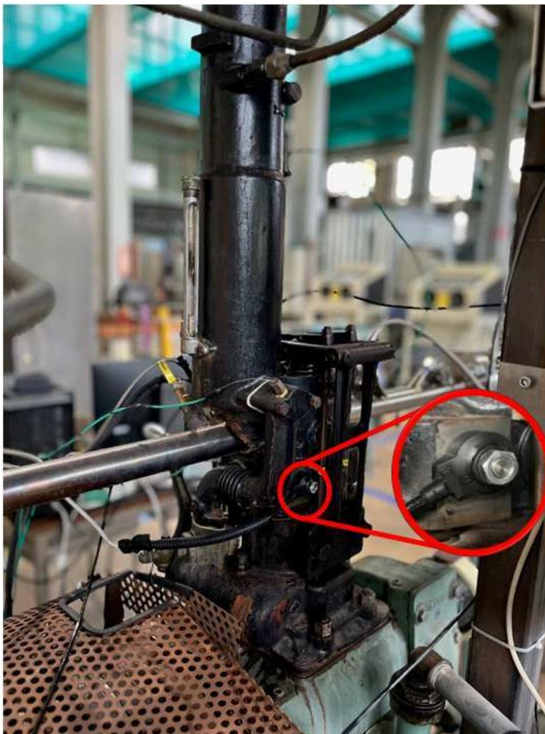
*Figure 6.2: Mounting location of the knock sensor on the CFR engine.*
