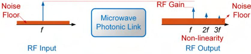
Figure 4.3: The figure of merit of a microwave photonic link.
