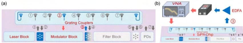
Figure 7.11: Optical transmitter characterization. (a) Sample configuration as an optical transmitter. (b) The setup for the measurement. VNA: Vector Network Analyzer; PD: Photodetector. SiPh sample: Silicon photonic sample. EDFA: Erbium-doped fiber amplifier.
