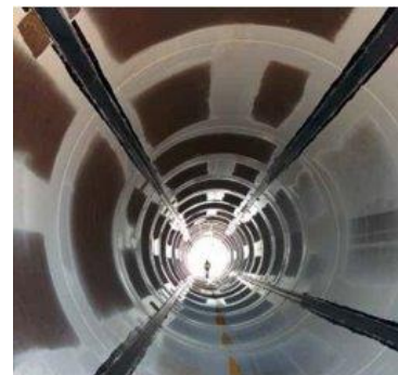
Figure 1. Inside view of an instrumented monopile, black lines are optical fibres on which the FBGs are mounted at different depths.
