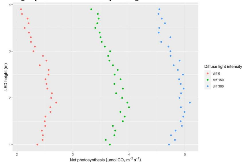
Figure 1. Net full plant photosynthesis simulated for different intensities of diffuse (diff) solar radiation. In each simulation (represented by the individual points), the crop is supplied with HPS toplighting and one LED light bar at varying heights (y-axis).
