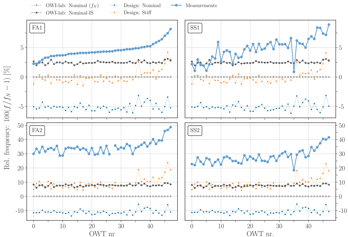
Figure 2. Comparison of measured frequencies, as-designed frequencies and frequencies computed with the integrated OWI-lab FE model. All frequencies are expressed relative to the corresponding nominal frequencies computed with the OWI-lab: Nominal model, and have been sorted such that the error between the measured first fore-aft frequency and the corresponding nominal frequencies are in ascending order. Upper half: first order fore-aft and side-side frequencies. Lower half: second order fore-aft and side-side frequencies.
