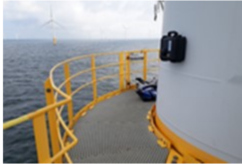
Figure 1. Mobile measurement system containing accelerometers.
