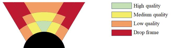
Figure 5: Quality category is assigned based on distance and field of view.
